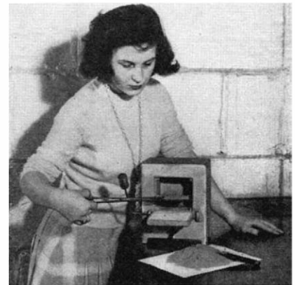
A small electric furnace is part of the equipment for diamond-dust recovery
