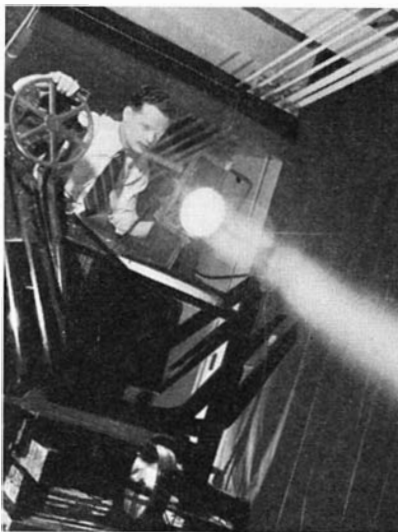
War-born successor to the sealed-beam automobile headlight, rated at 600 watts, is here being tested to determine its ability to light up runways
