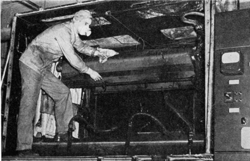
Lighting fixtures are tested for over-heating and dust-tightness in this dust chamber. Dust-tight fixtures are designed for use in hazardous locations in dusty factories where an exposed spark or flame may set off a disastrous explosion
