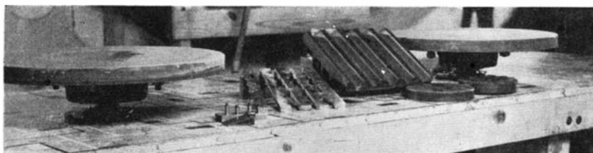
Figure 2: Fogarty's grinding spindles (splash-plates removed)
