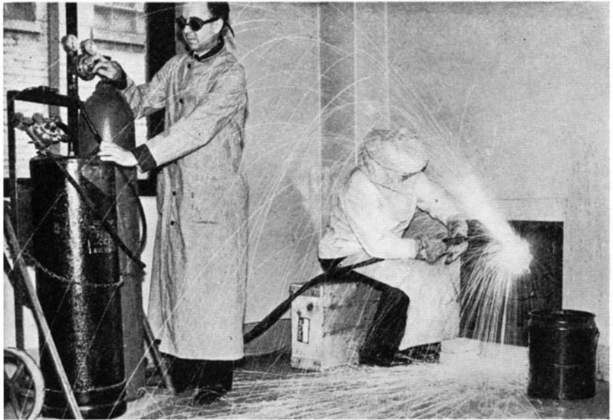
A torch attack on a vault door in which is installed a microphone burglar alarm intended to detect noise of such attacks and send an alarm. Underwriters' Laboratories has made a series of recordings of the noises made in carrying out various types of attacks on vaults. With these recordings many burglar-alarm systems can be accurately tested
