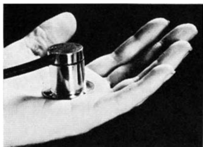
One of the electric ears used in the detection of aircraft vibration
