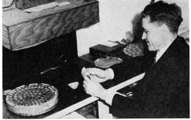
Sandy MacTavish and the unpretentious back-yard shop in which he and Pavel Uvaroff produce pretentious roof angle prisms. On the bench are two 97-prism polishing matrices and a flat for testing them by interference fringes (light source above)
