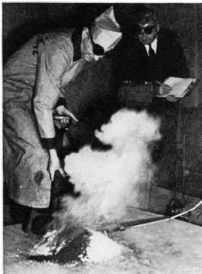
Testing materials for extinguishing magnesium fires at Underwriters' Laboratories. Thermocouples are placed in the center of the pile of burning magnesium; temperatures are read from recording instruments in background. Efficiency of extinguishing material is determined by speed of reduction of temperature
