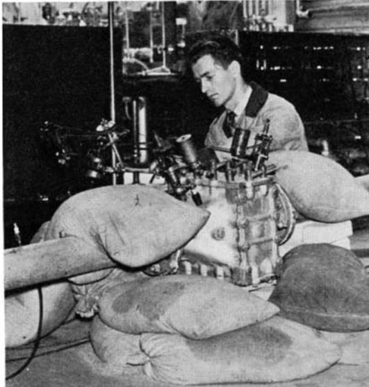
Flame arresters for vent lines of oil storage tanks are tested with this equipment. The arrester is placed in the line shown and gas mixture introduced into each end. One explosive mixture is fired; a few seconds later the other is touched off. If the second one explodes, it proves flame from first did not pass arrester
