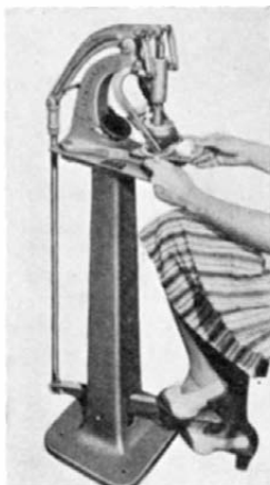
Rubber, cork, plastic, felt, fiber, and other parts may be successfully printed on this machine
