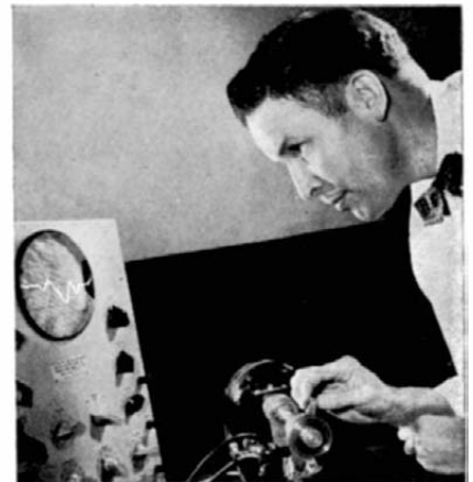
Electronic fingerprints — A Westinghouse Research Engineer demonstrates the principle of the electromagnetic flaw-detector. Hard spots in the steel test piece show up as an irregular line on the oscilloscope screen.
