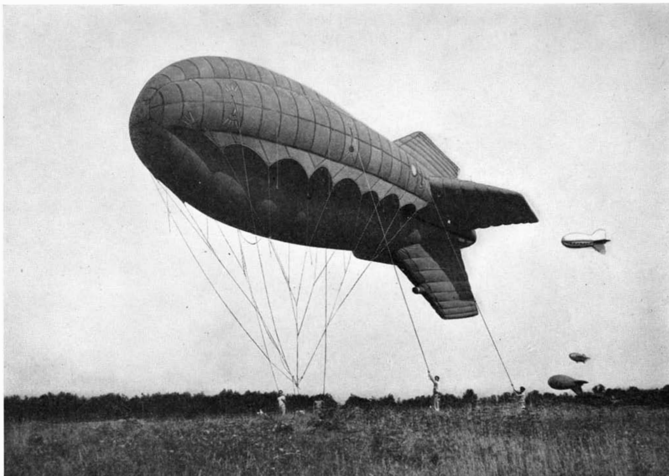
"Staking out" a four-lobe barrage balloon where housing facilities are not available
