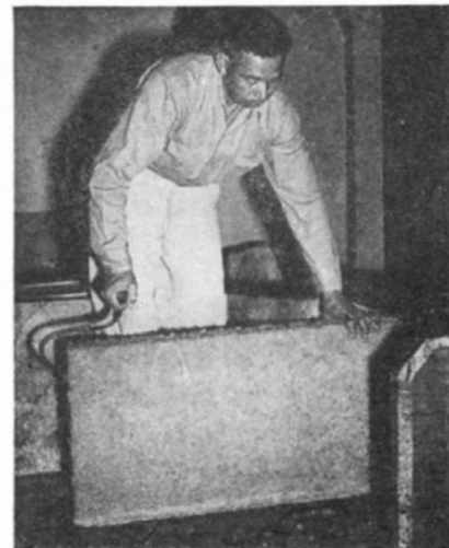
Introducing 100-pound block of frozen agar gel into a chopper which grinds the gel to small particles
