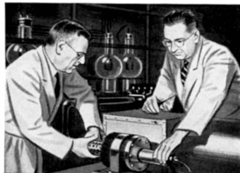
1937. Bloomfield, N.J. Westinghouse developed the key electronic tube for the U. S. Army's first Radar equipment used to detect aircraft. Radar focuses invisible, ultra-high-frequency waves traveling at 186,000 miles per second.
