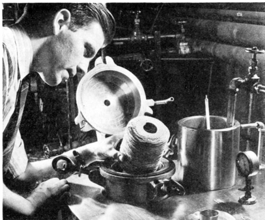
Much yarn is dyed in what are known as "packages." These are steel bobbins wound with yarn which are placed over circular tubes in a cylindrical machine and the cover bolted in place. The dye liquor is pumped through the tubes and forced out through the yarn. Shown is a laboratory package dyeing machine which is, in every respect, a small-scale duplicate of its counterpart used in commercial production
