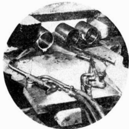
Steel solenoid housings and saddles are cleaned and fluxed, then assembled with a thin strip of silver brazing alloy between them. Heat is then applied, as shown, to melt the alloy and complete the joint
