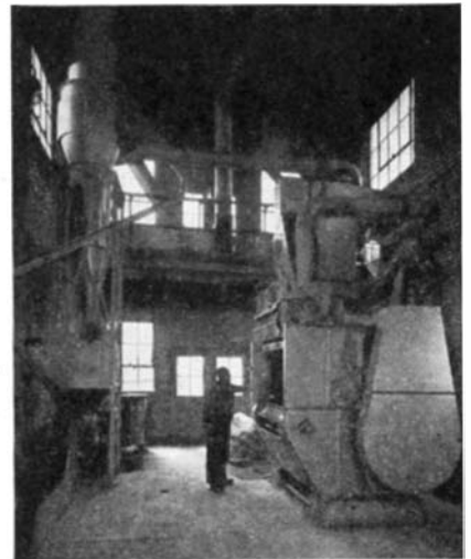
A shot-cleaning machine is sealed dust tight and a cyclone removes the dust as fast as it is produced
