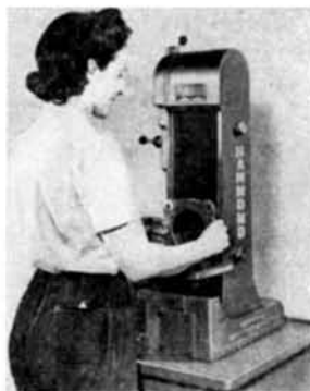
Belt grinder which can be adjusted from vertical to horizontal while running
