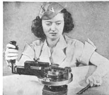
BENDERS —DI-ACRO Bender bends angle, channel, rod, tubing, wire, moulding, strip stock, etc., 2 sizes. Capacity up to \frac{1}{2} " cold rolled steel bar.
