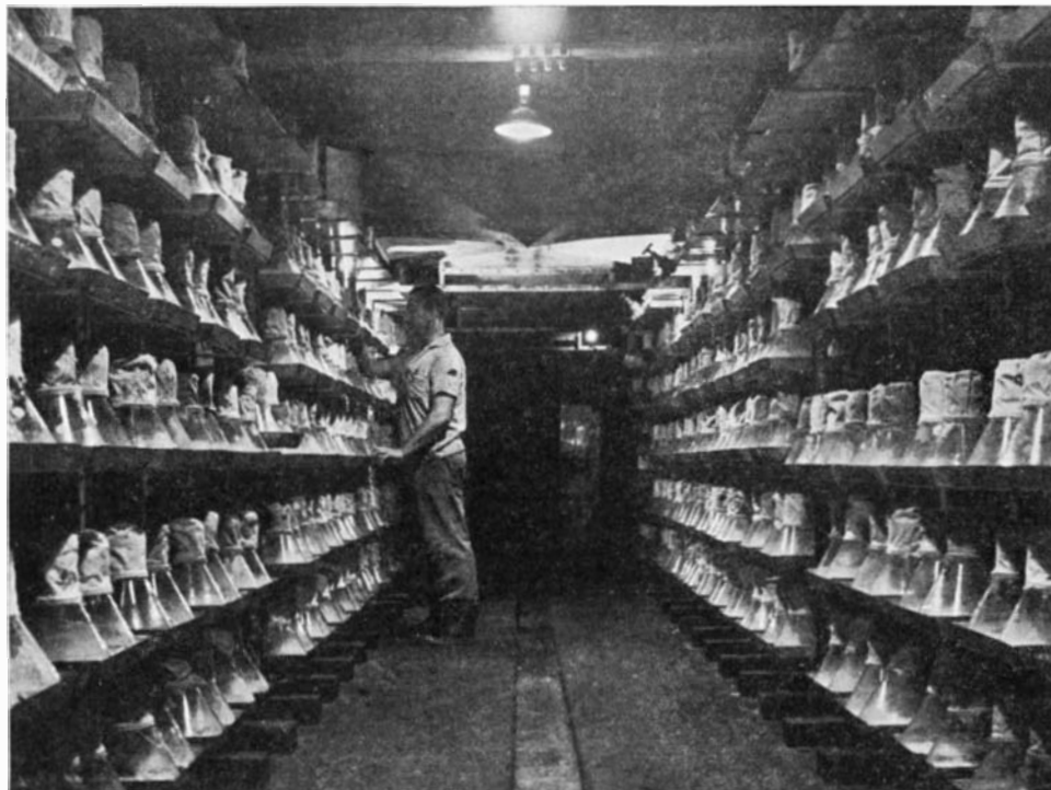
Illustrations not otherwise credited, courtesy Chas. Pfizer and Company In the flask fermentation room of a penicillin pilot plant
