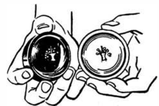
Fine detail easily recorded in the alloy sprayed onto pattern.
