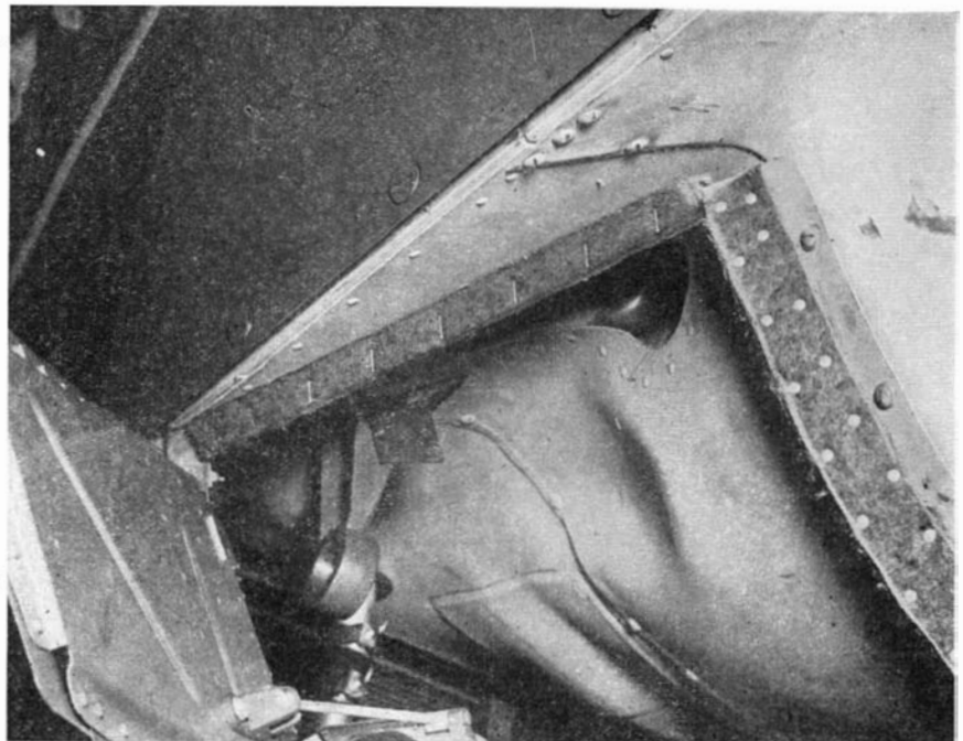
Two methods of fastening strips of wool felt to metal. Right: Felt sealing strip fastened by old method of riveting. Left: New Morrison metal stitcher method
