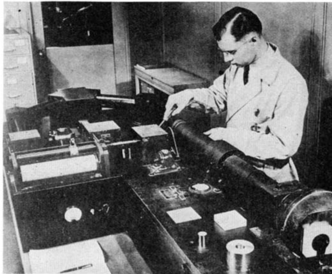
Recording photoelectric spectrophotometer made by General Electric in the laboratory of Interchemical Corporation, where it is used to establish color for inks, paints, enamels, and so on
