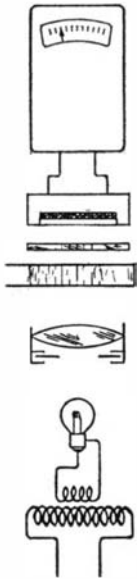
Diagram, very much simplified, of a typical photoelectric colorimeter
