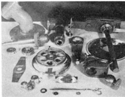
Figure 2: Details of mounting. For rough, temporary end-nut in first photograph substitute streamlined version in second
