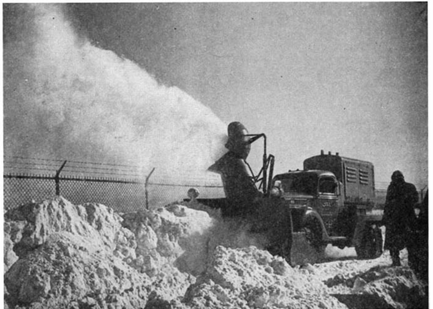
Rotary snow throwers dissipate snow piled up by plows
