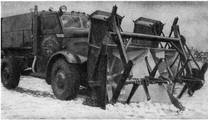
The rotating forks at the front end of this machine break down any kind of snow bank and feed it to blowers which throw it well off to one side
