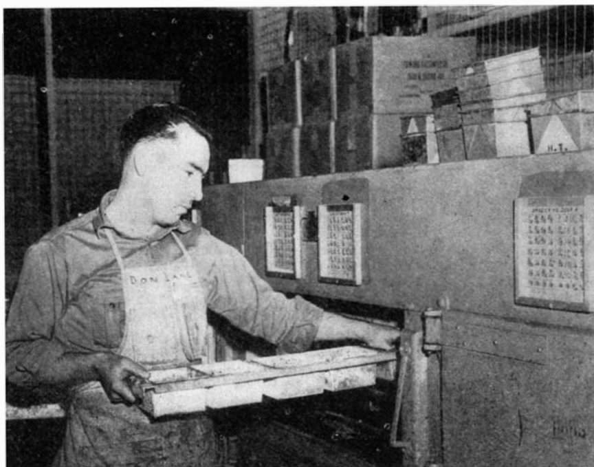
Refrigerators at a Douglas aircraft plant keep aluminum rivets cold and soft
