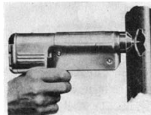
Blind rivets may be driven rapidly with this light-weight pneumatic tool
