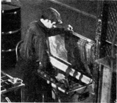
Portable containers, refrigerated by dry ice, are used to distribute aluminum rivets throughout a factory
