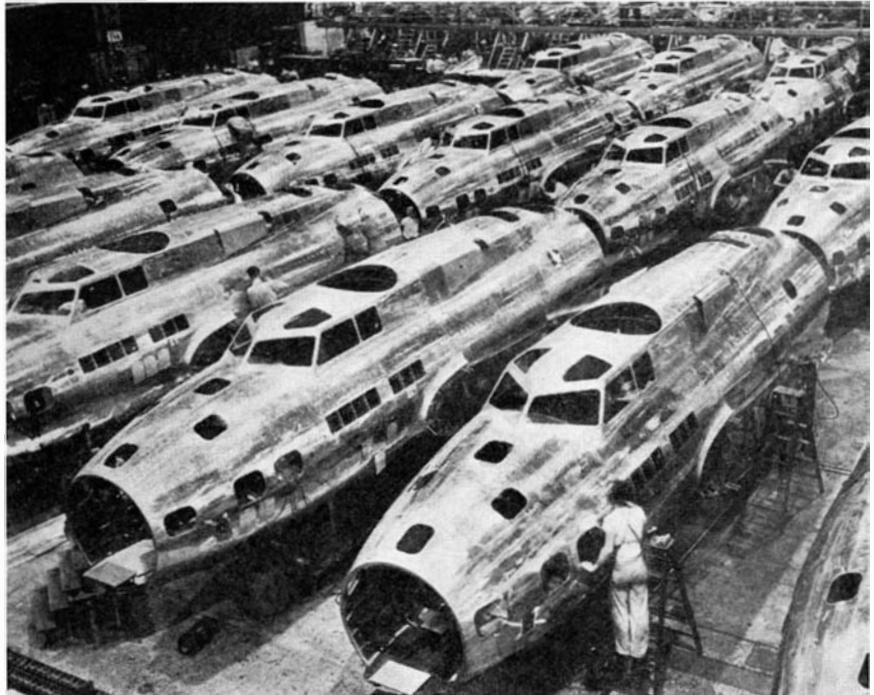
Main fuselage sections of Flying Fortresses advancing on the production line
