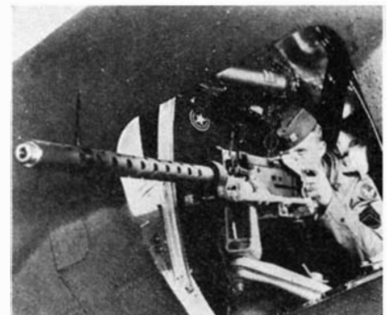
Above: The light-weight cradle of the hydraulic gun-recoil device described in the accompanying note. Below: The waist gunner of a Martin B-26 Maurader lining up a target by the use of the new absorption unit
