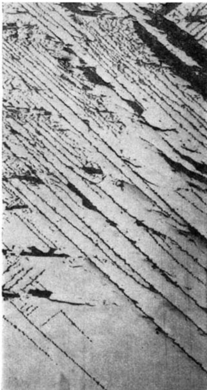
These plastic flowlines on steel after permanent deformation tell us a tale
