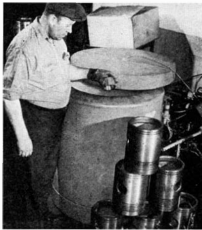
Rapid assembly of bronze piston bushings is accomplished by chilling the bushing prior to insertion
