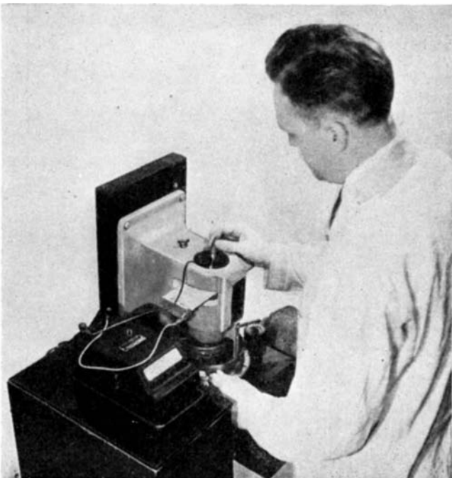
Testing paint-film flexibility with the Elongage, described in the text. The panel under test may be seen in the device
