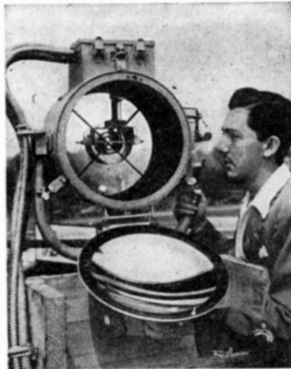
New arc searchlight, with back removed
