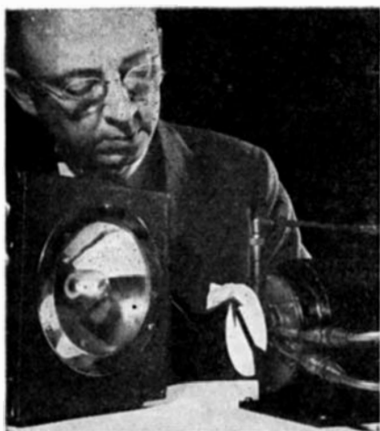
Ultra high-speed motor—a veritable "whirling dervish"—being speed-checked with a stroboscope
