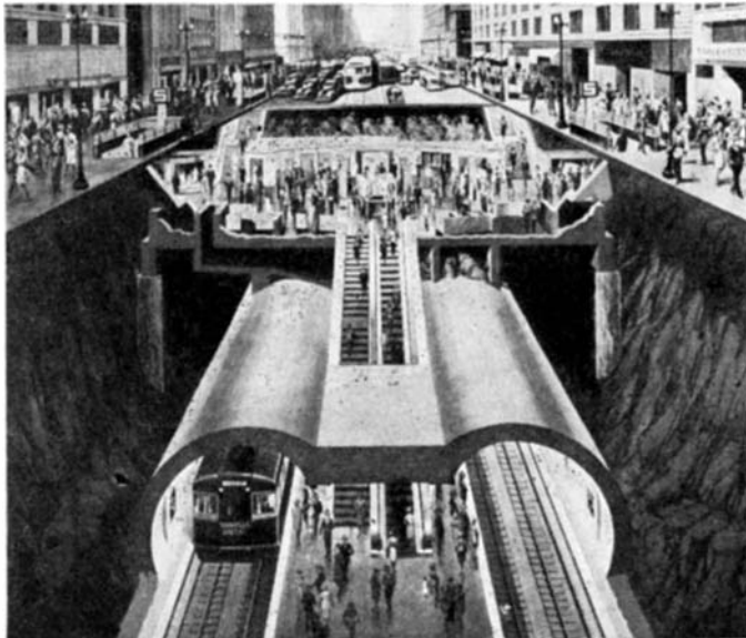
Stairs lead from sidewalk entrances of the Chicago subway to mezzanine stations; escalators and stairs lead to platforms
