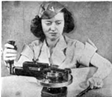
BENDERS —Di-Acro bender bends angle, channel, rod, tubing, wire, moulding, strip stock, etc., 3 sizes. Capacity up to ½" cold rolled steel bar.
