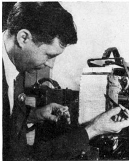
A dab of red paint shows on the improperly charged fuse, which was also detected on the meter graph
