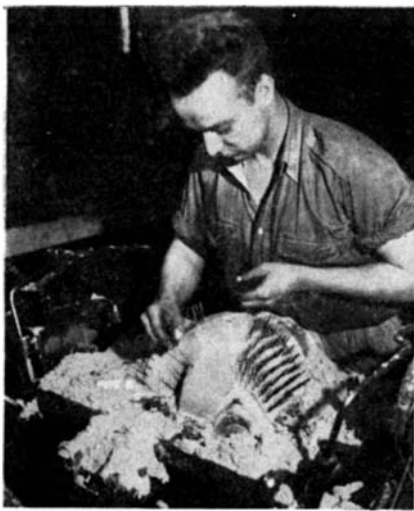
Courtesy Wright Aeronautical Corporation Making a mold for casting an aluminum cylinder head for an aircraft engine. Long nails are inserted into the sand to act as reinforcements during pouring of the metal
