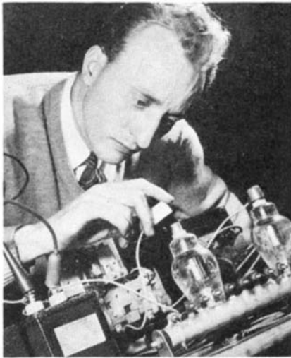
Interior of an energy storage welding control made by Westinghouse and used for welding aluminum parts
