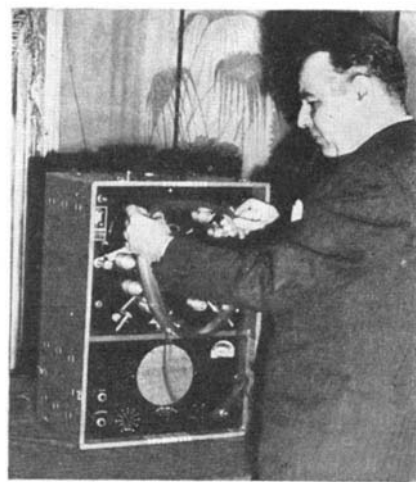
Eight hours of continuous sound can be recorded on the cellophane loop being loaded in the recorder
