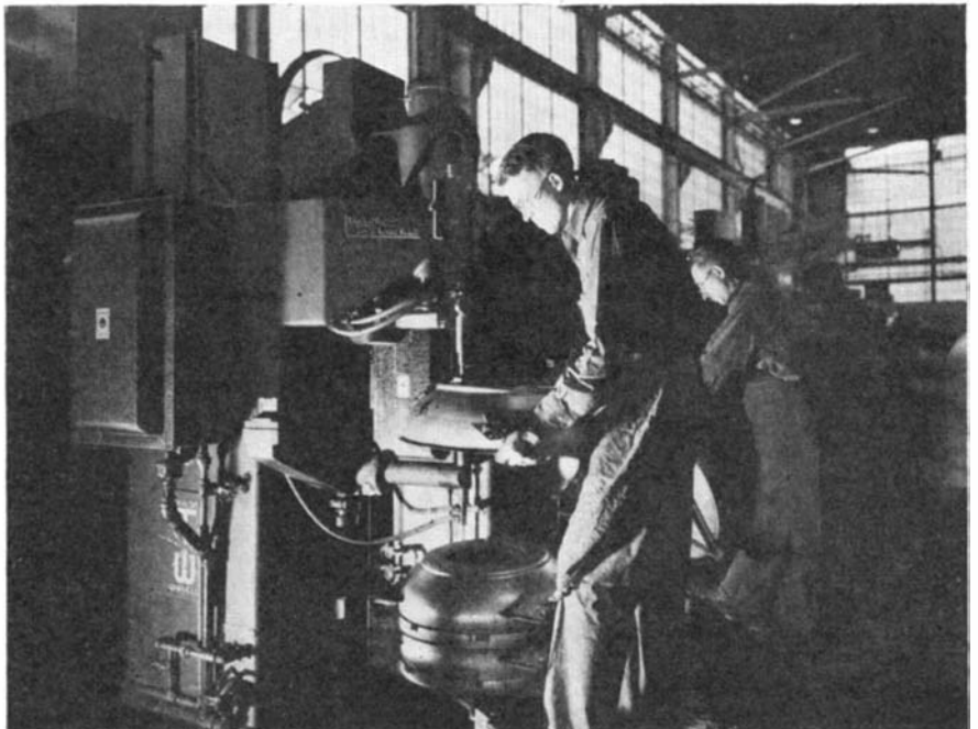
A sequence timer controls current and strokes per minute on this spot-welding job
