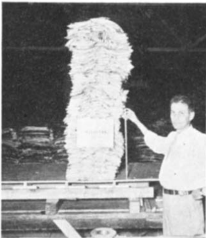
Weight test of new floor panels
