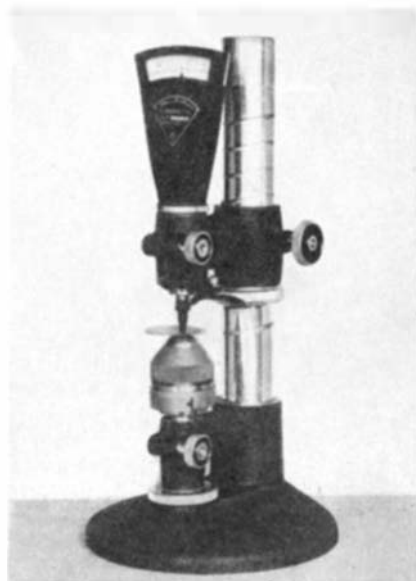
A radio quartz crystal, only .030 inch thick, being gaged between a flat spindle and spherical anvil
