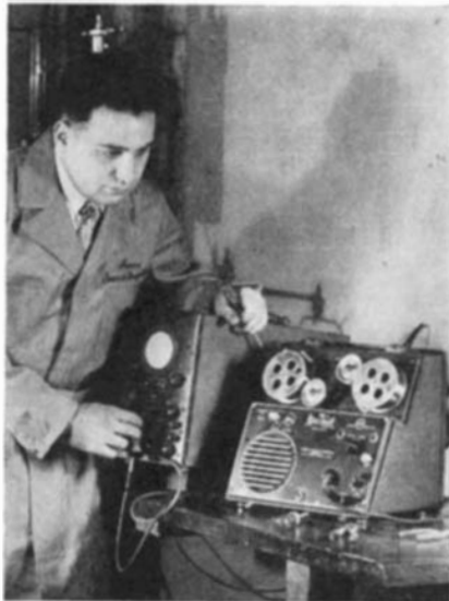
Checking the frequency response of new magnetic wire sound recorder
