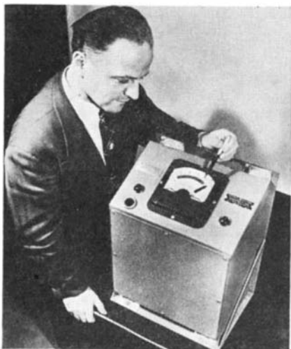
Safety margin in crane operation is indicated by this new instrument
