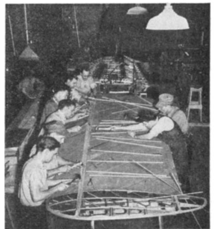
The plywood skin of an airplane wing panel being applied in one of the Fairchild aircraft plants
