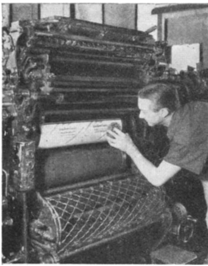
Washing-up a plastic printing plate
