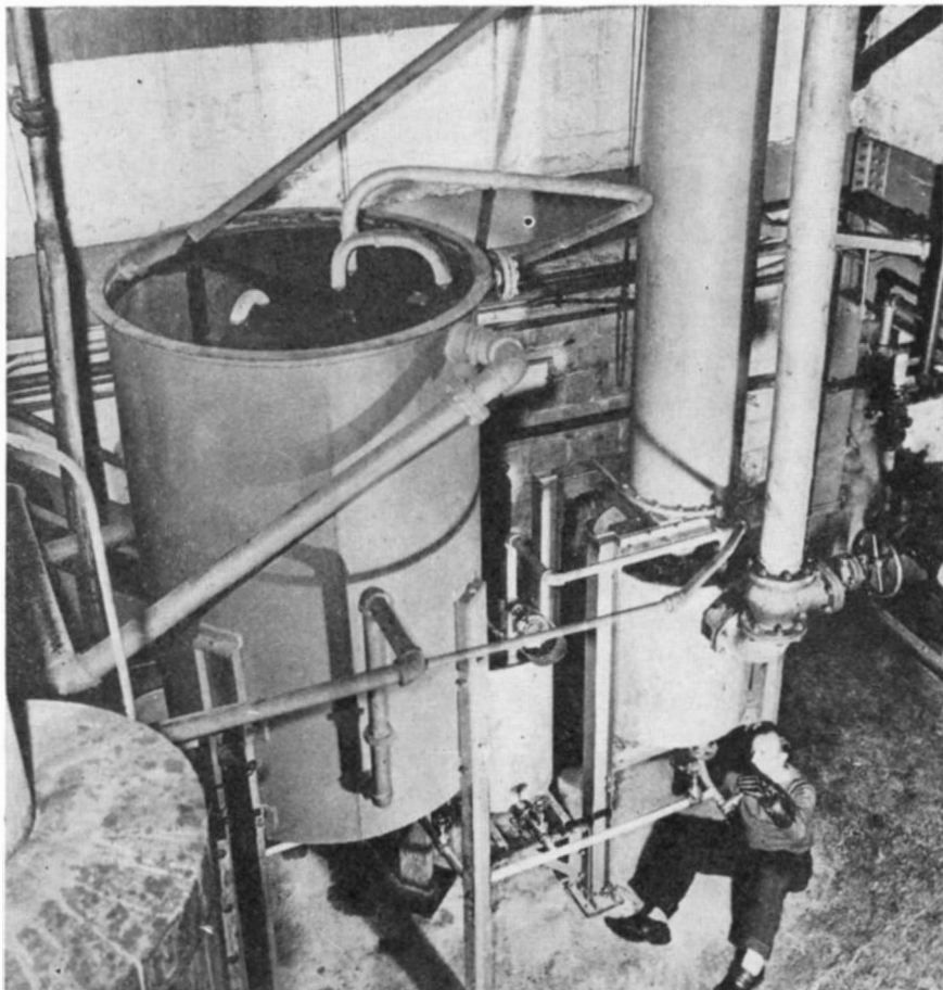
In this equipment, in a plant of the Woburn Degreasing Company, castor oil is processed to obtain a drying oil that will replace tung oil in surface finishes
