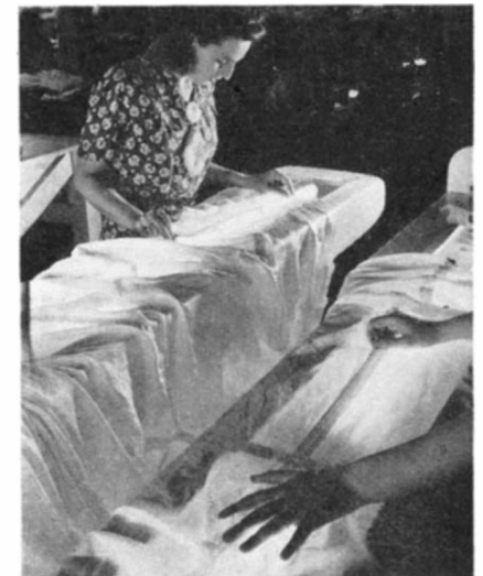
Illuminated tables speed inspection
