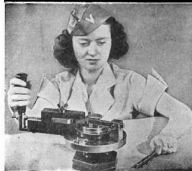
BENDERS —Di-Acro Bender bends angle, channel, rod tubing, wire, moulding, strip stock, etc., 3 sizes. Capacity up to 1/2" cold rolled steel bar.
