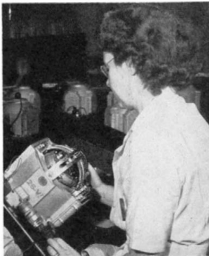
Spinning gyroscope unit of an electronic automatic pilot being tested on a tilt table at a plant of Minneapolis-Honeywell Regulator Company
