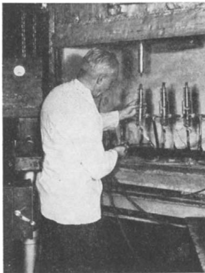
During manufacture, X-ray tubes are tested in this cabinet, which is lead lined to protect the operator
