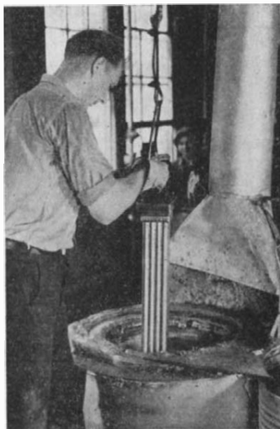
Removing a steel pattern from the molten lead bath used in the manufacture of molds for casting plastics. The lead is later reclaimed
