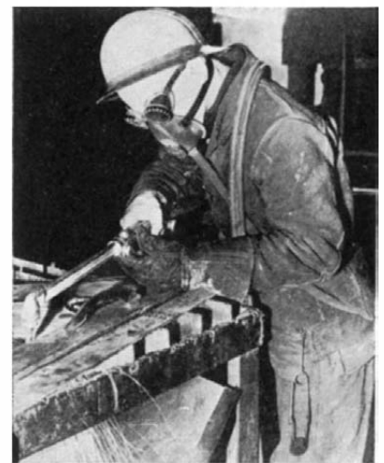
A light chipping operation requires protection for face, hands, and trunk
