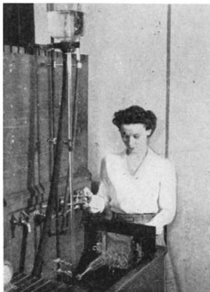
Testing water repellency of fabric
