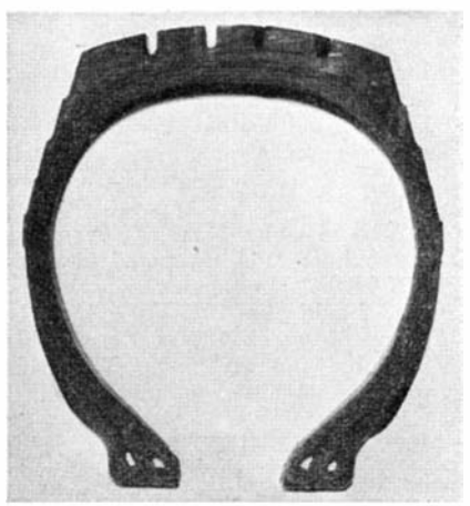
Cross-section of the new truck tire, showing shoulder ventilating grooves
