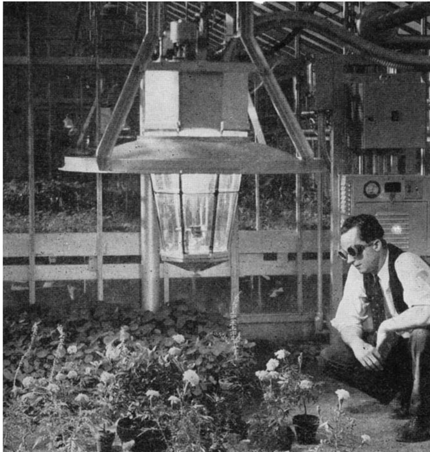
In this pest-control research laboratory maintained by Du Pont, actual field conditions are closely paralleled. The light from the large lamp simulates sunlight
