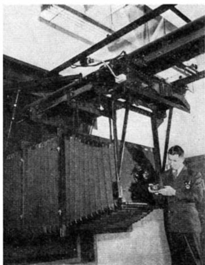
Steel girders support the photo-template camera and connect it to easel, insuring complete rigidity
