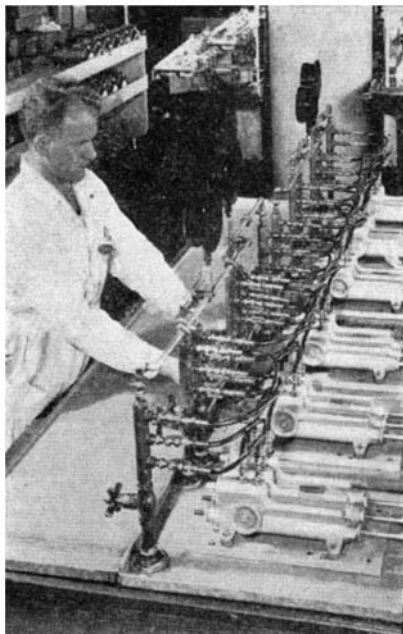
Above: Hoses made of a synthetic resin are important parts of this stand for testing automatic pilots. Right: These flexible hoses withstand hydraulic pressure and flexing
