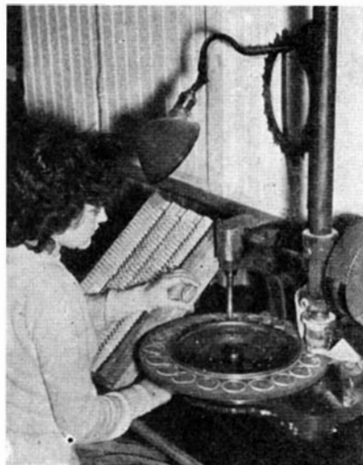
Testing safety lenses for toughness. As each lens is positioned under the pipe column at the right, a 5/8-inch steel ball weighing over half an ounce is dropped from a height of six feet and strikes it
