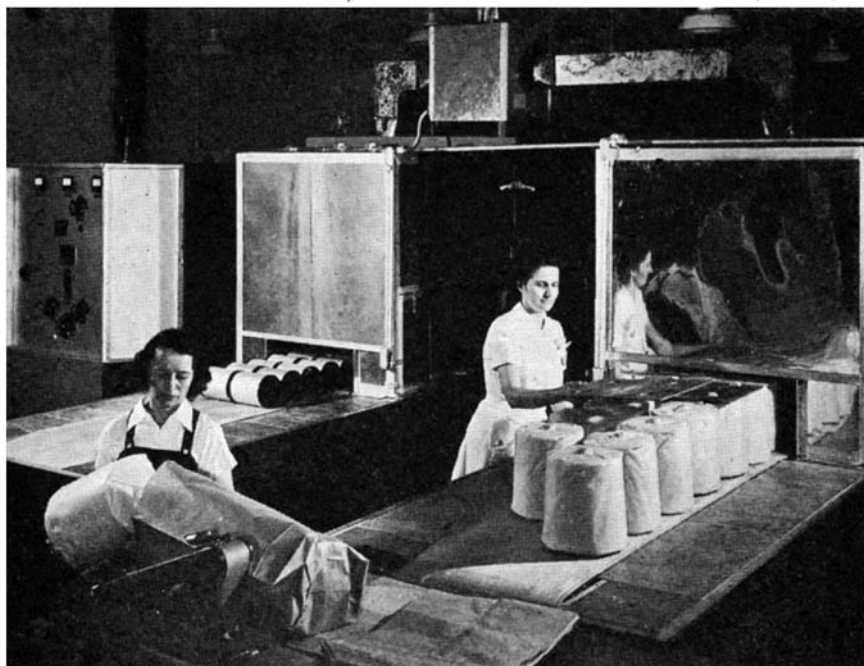
Twist of rayon tire cord, in 18 pound cones, is set in electronic heater at right
