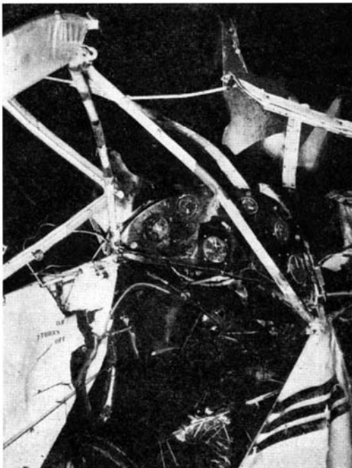
Figure 2, left: A fatality was recorded in an airplane accident when the pilot's head struck the diagonal brace shown, bending it and fracturing his skull. The passenger in rear was uninjured
