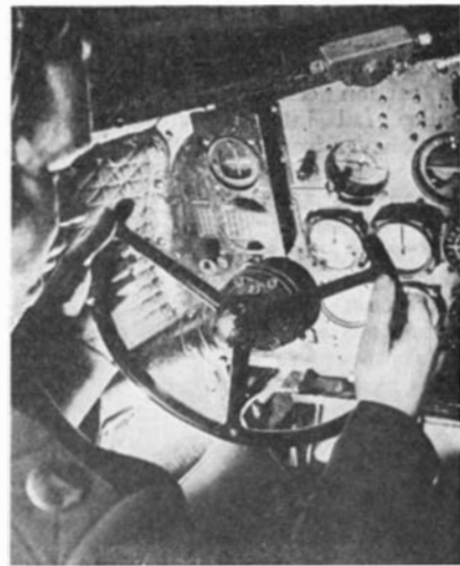
Above: Checking blind-landing instruments. The third unit from left shows correct position of pointers when landing. Below: The blind-landing instrument is on the panel just above the pilot's control post
