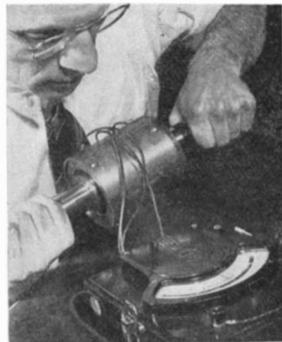
The torquemeter is sensitive enough to measure the degree of twist exerted in a steel shaft by the hands
