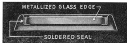
Sprayed copper permits soldering
