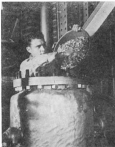
Courtesy Northern Regional Research Laboratory Cornstalks being placed in a digester as first step in plastic making
