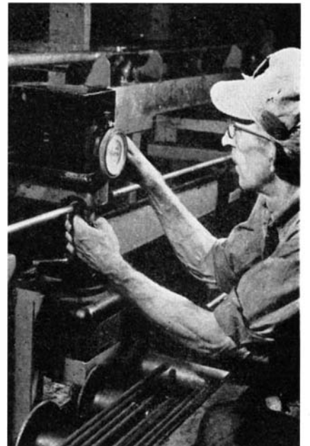
Below: Every fifth heat-treated bar is checked for Rockwell hardness
