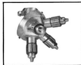
Quadrill assembly complete ready for attachment to drill press
