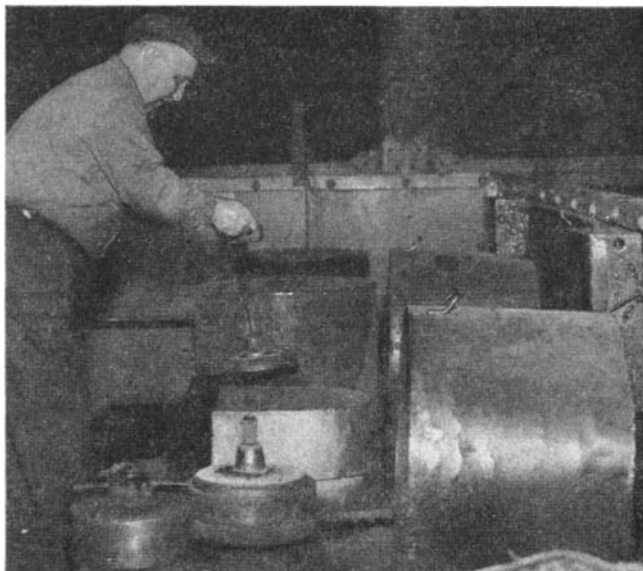
Removing a centrifugally cast gear blank from one of the casting machines shown in the illustration at the left
