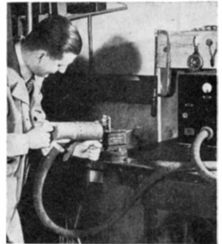
This RCA electronic detonator of explosive rivets is being used in aircraft plants to speed up assembly work. High-frequency currents generate sufficient heat to detonate small charges of explosives in the rivets, spreading them at the end
