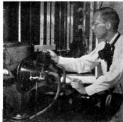
An automatic pipe smoker being used to check the efficiency of filters
