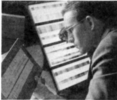
Spectrograms made by the light radiated from a bar of ultra-pure iron as it glows under the heat of an electric arc (above), are compared (right) with wavelength "portraits" of other metals for checking quality
