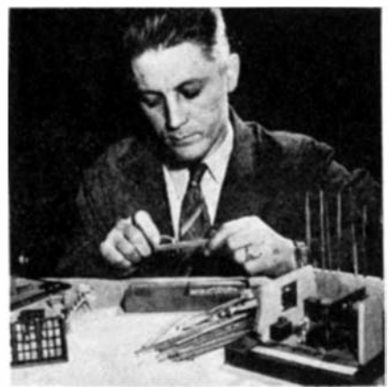
Even routes for roller conveyors are determined in miniature by engineers using "industrial doll-houses"
