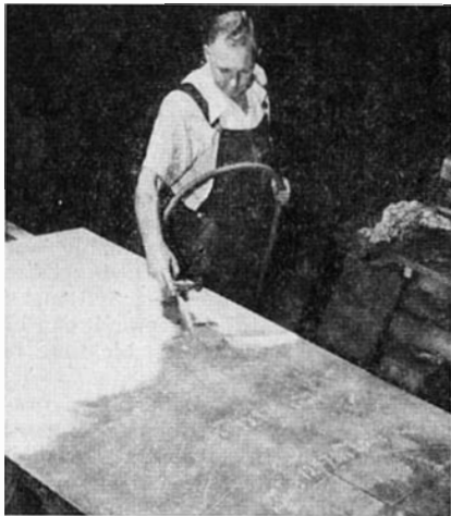
A spray of tap water removes all layout paint which has been light-struck, leaving only the lines and figures of the original drawing
