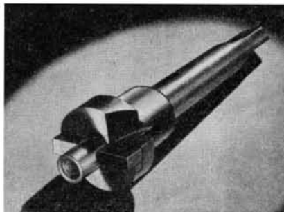
The bit is locked with set screws
