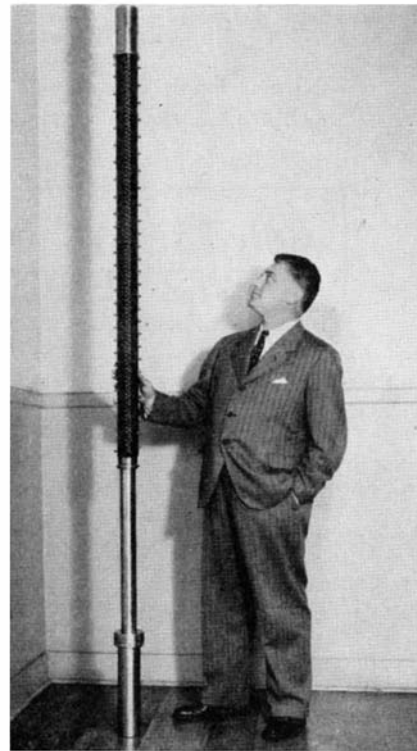
Mr. R. R. Machlett with the new precision high-voltage x-ray tube developed in Machlett Laboratories
