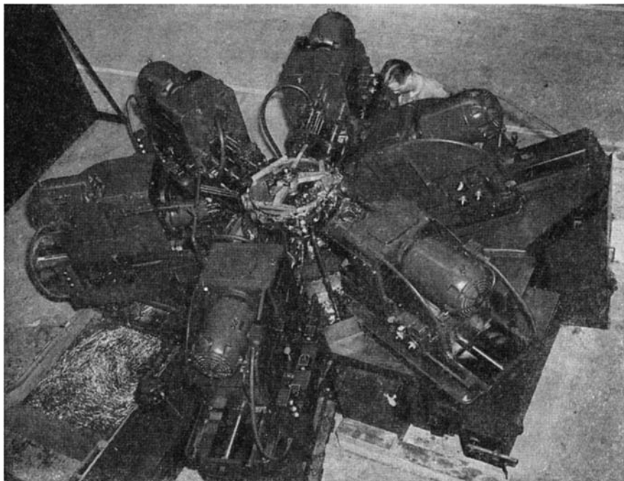
Figure 2: This Greenlee six-way horizontal automatic machine performs a number of simultaneous operations in the front section of a supercharger
