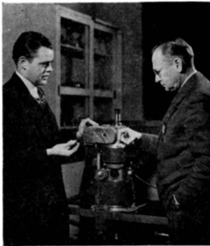
Drs. Zworykin (right) and Hiller, of RCA Laboratories, with an experimental model of the electron micro-analyzer, latest of the electronic research tools for industrial scientists
