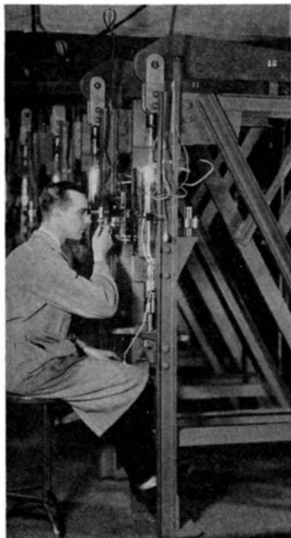
Creep tests being conducted in the research laboratories of the United States Steel Corporation. Such tests as these are part of the development program that has given rise to new heat-resistant alloys for gas turbine and supercharger components
