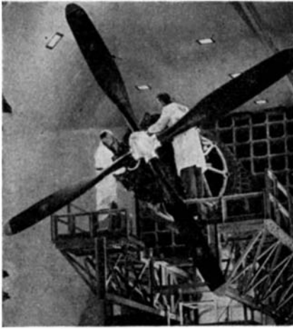
Preparing a 16-foot, 8-inch, diameter propeller for testing in a Curtiss-Wright propeller-research test cell
