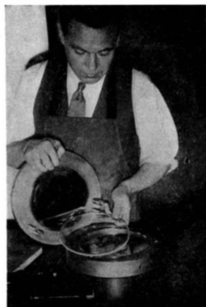
Removing from its mold one of the plastic lenses used for projecting brighter, larger television images
