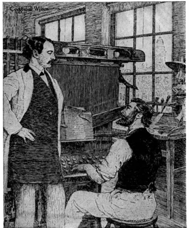
Otto Mergenthaler demonstrating the operation of the "blower machine," the first successful linotype, for Whitelaw Reid in the plant of the New York Tribune
