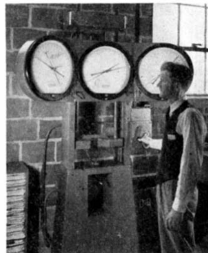
Courtesy Rustless Iron and Steel Corporation Checking tensile strength of steel
