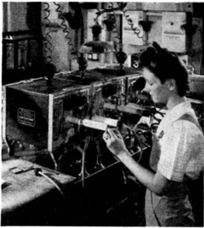
Courtesy Rustless Iron and Steel Corporation Carbon determinations by the laboratory control the quality of steel
