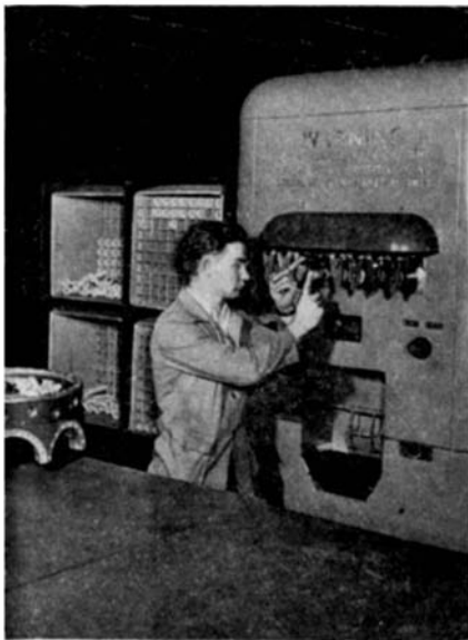
A tappet guide insert at room temperature is pushed into the freezing dispenser. Cold-shrunk inserts are delivered, as needed, at the bottom
