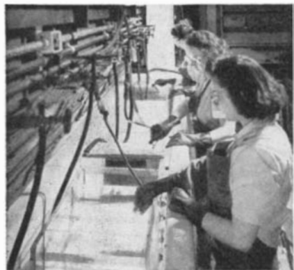
Non-corrosive glass tanks, designed for Westinghouse by Pittsburgh Plate Glass as a war-time substitute for metal and wood tanks, are found better in many ways than old types
