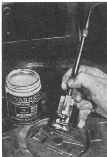
Worn parts and shafts may be renewed with this electrolytic brush
