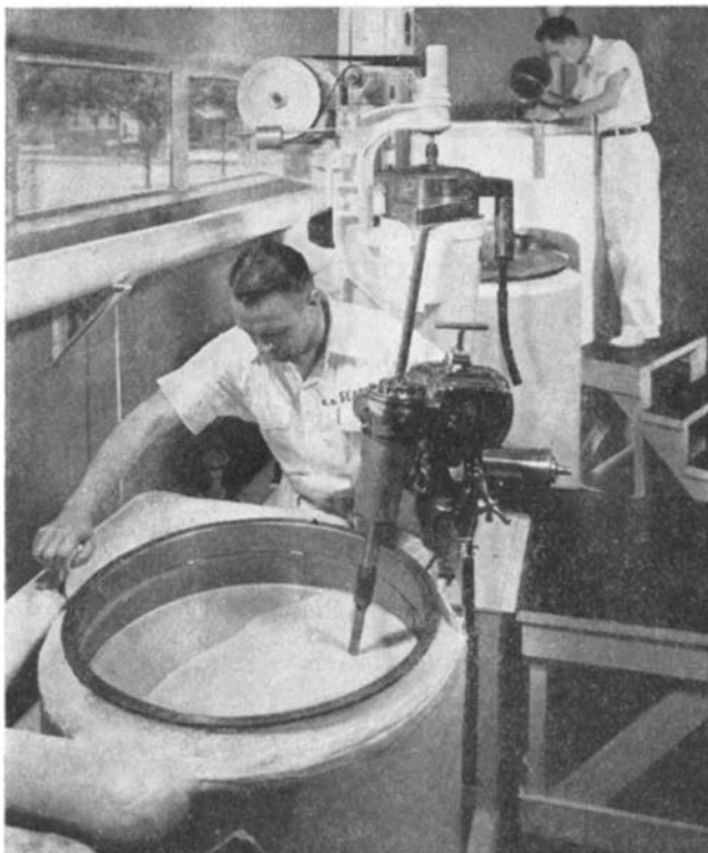
Portable mechanical mixers play a large part in the efficient operation of pilot plants and in small-batch work
