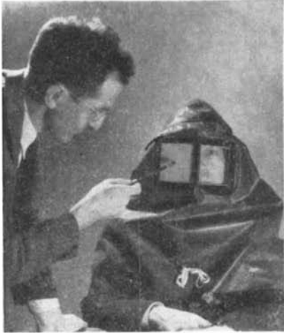
One of the lenses in this worker's hood is of ordinary glass; the other is resistant to hydrofluoric acid. Note how acid has etched lens on left
