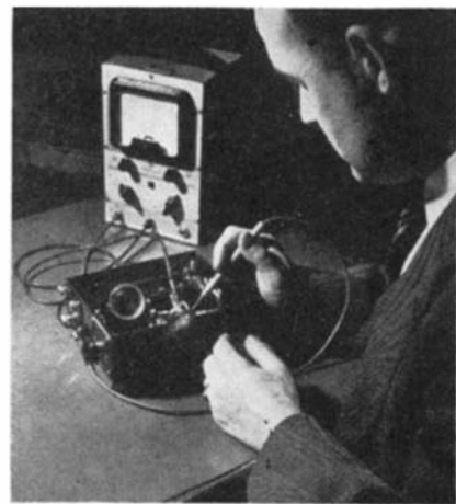
Photocell in the x-ray timer measures light on fluorescent screen and controls length of exposure
