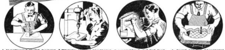
1. PAINSTAKING CENTER PUNCHING 2. TEDIIOUSLY DRILLING ROW OF HOLES 3. HAMMERING OUT THE SLUG 4. FILING OFF THE DRILLMARKS
