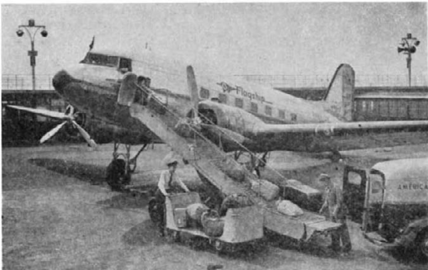
Adjustable for height, the conveyor belt is powered by a tractor engine
