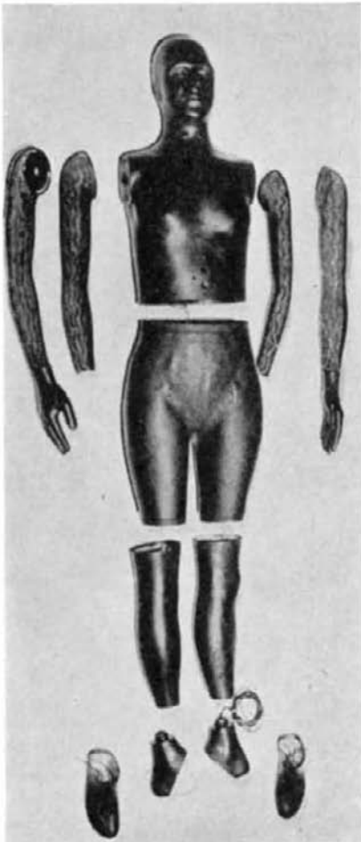
Parts of the "copper man," which reproduces human body temperatures for laboratory research on clothing
