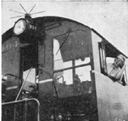
Radio enables the engineer of this Baltimore and Ohio switching engine to receive his orders. The antenna of the receiver-transmitter is seen on the cab roof over the headlight
