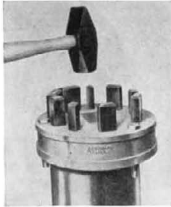
A single blow marks the work
