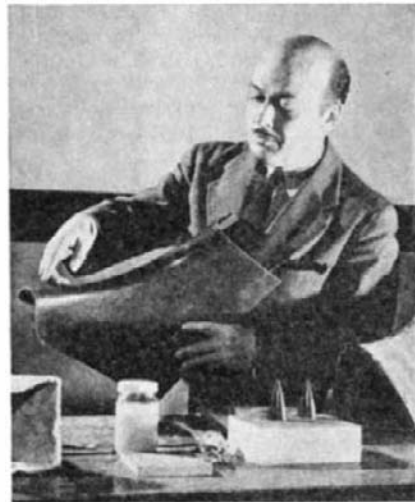
An airplane tail fillet made of new light but strong preformed plastics
