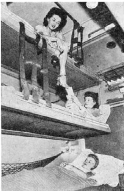
Above: Solid comfort in the three-tier sleeper the railroads plan to introduce for lower-income travelers. Lower right: During the day the new sleeper will be divided into seats set three in a row across the car. Lower left: At night the car will be made up so that each triple tier of berths will divide into a section
