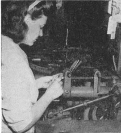
An operator threads wire through one of the several diamond dies on a modern power-driven wire drawing machine
