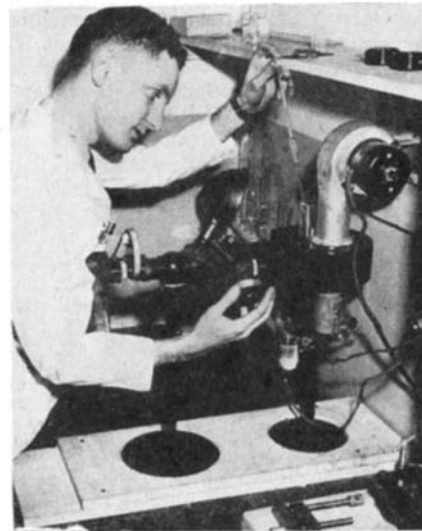
Pipetting a sample of a test solution into the chamber of the turbidimeter
