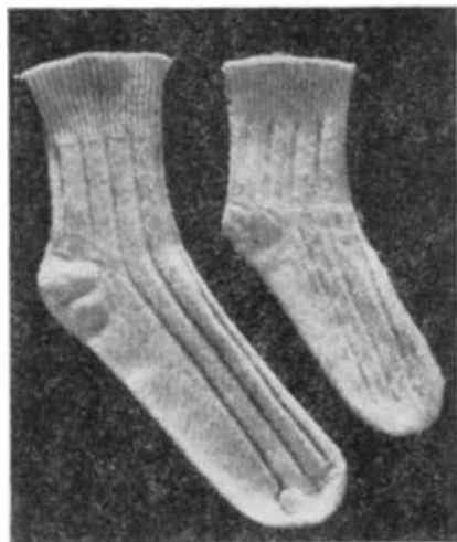
Two hours in soap and water did not change the sock treated with Lanaset
