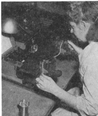
Ohmage of resistance wires is accurately checked on a Wheatstone bridge
