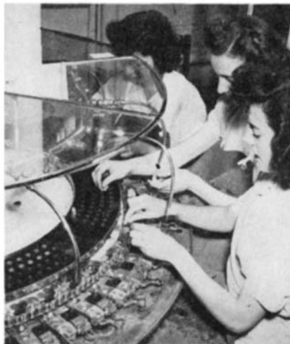
Above: Special clips hold different size filters on the conveyor belt of the automatic laminating equipment. Right: Placing filter blanks between glass. The resulting "sandwiches" then go to the automatic laminator
