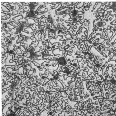
Figure 1: An alloy of 80 percent copper, 10 percent tin and 10 percent lead.
