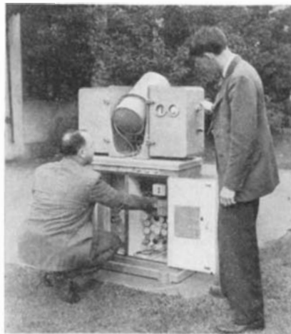
The new G.E. ceilometer obtains cloud ceiling data valuable to all aviation
