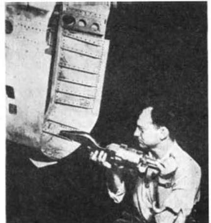
Compressed air squeeze riveter at work in speedy aircraft fabrication
