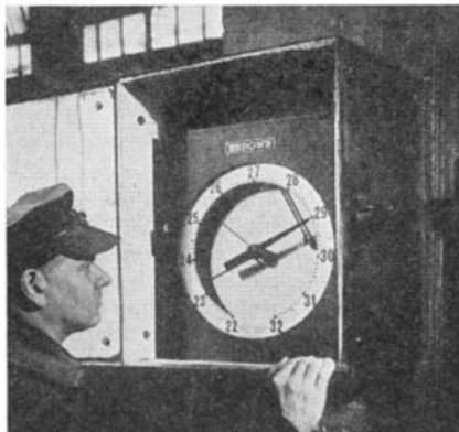
A worker checks the big dial of the electronic device which records temperatures ranging from 2200 degrees up to 3200 degrees, Fahrenheit, at the Rustless Company's Baltimore plant
