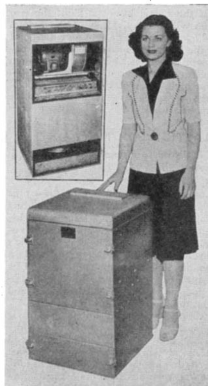
Filters (inset) remove dusts that arise in many industrial operations
