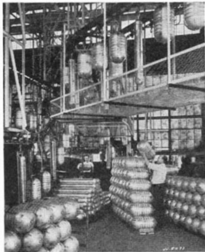
Production line for non-exploding oxygen cylinders made of stainless steel
