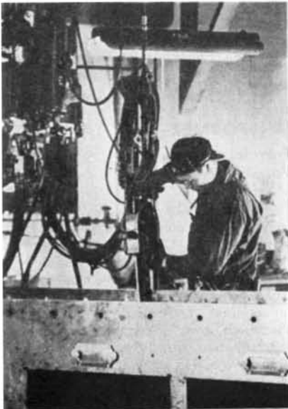
A spot-welding gun, suspended above the work, solves production problems
