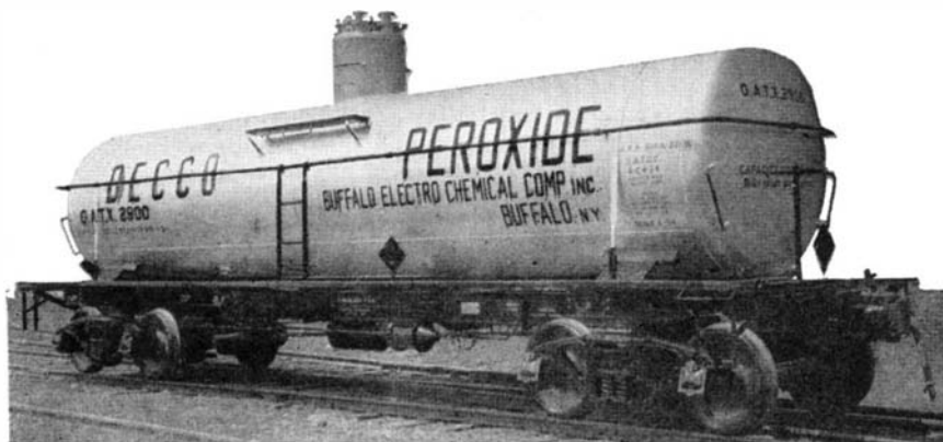
An all-aluminum welded tank car designed for transporting peroxide
