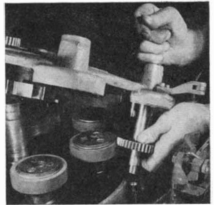
Synthetic rubber rings, meshing with metal gears, provide positive transmission and give long service life
