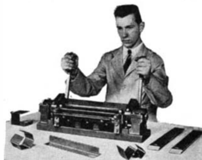
Fracture of low ductile metals is almost impossible with this brake
