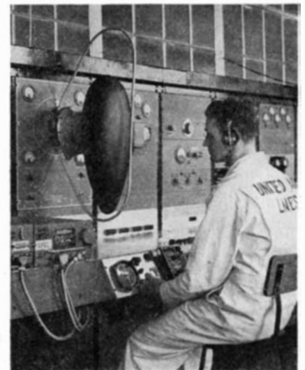
Automatic direction finders are checked for accuracy before installation in an aircraft. The blimp-shaped casing to the left houses the antenna
