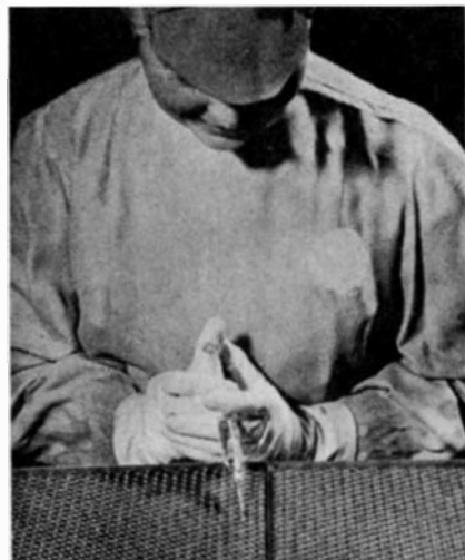
A hypodermic syringe is used to put a drop of oil in these tiny bearings. White gloves, gown, and cap worn by the operator safeguard against dirt
