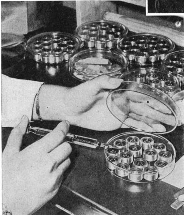
Flyers' lives often depend on their instruments. G-E workers use only tweezers to handle these precious parts of electrically driven gyroscopic instruments, dry them with air jets, oil them with hypodermic needles. They've got to be accurate.
