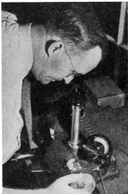
An engineer measures ten millionths of an inch tolerance in a bearing by the use of a microscopic gage of great power designed for this work
