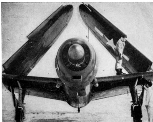
Folding wings, such as on Curtiss Helldivers, have greatly increased aircraft carrier effectiveness
