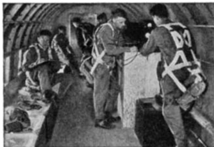
Sperry engineers testing intricate flight instruments in a “flying laboratory”
