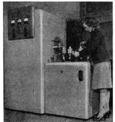
Simplified control and safety devices are features of this induction heater
