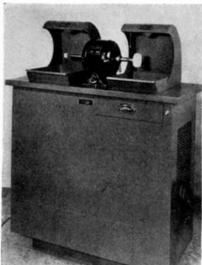
Filters and fan of this self-contained dust collector are in base
