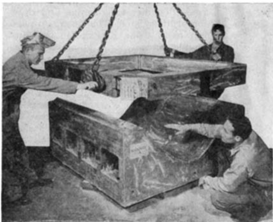
Two thirds of the weight of this huge die was eliminated by correct coring. It was made for use in the Douglas Aircraft Santa Monica plant
