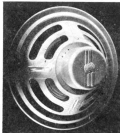
An Alnico permanent magnet acts as the heart of this radio loudspeaker
