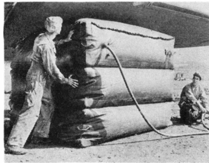
Photo by Air Technical Service Command Air pillows lift a plane
