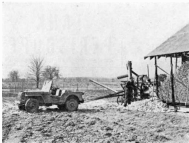
Versatile Jeep tows the corn husking machine to crib and is then put to work operating the long power belt
