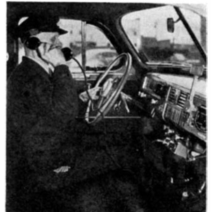
Right: Dashboard installation of a radiophone handset in a Cleveland cab. Left: Two-way radiophone equipment in the luggage compartment of a cab, showing the compactness of the 15-watt Motorola transceiver which has its own dynamotor (in foreground) for supplying the high voltages required by the radio tubes
