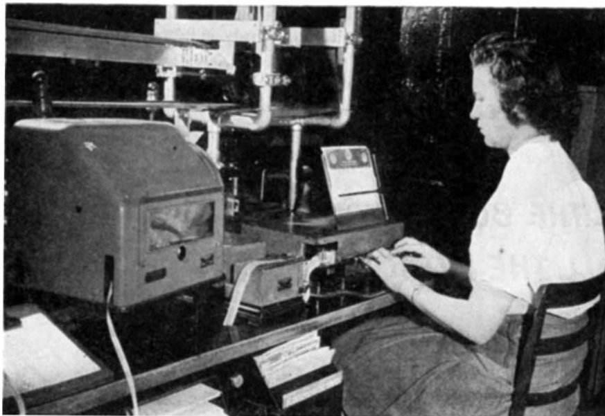
Punching tape for message transmission over eight-channel radio system
