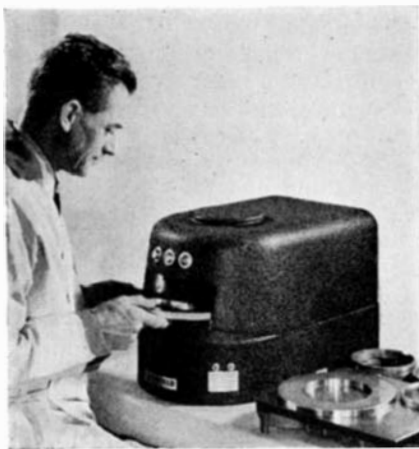
Quick gaging of piston rings
