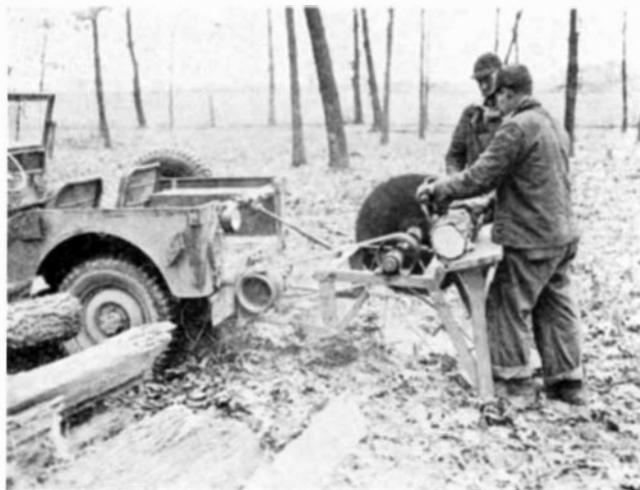
Taking the saw mill to the tree instead of the tree to the saw mill. The saw mounting folds into back of car
