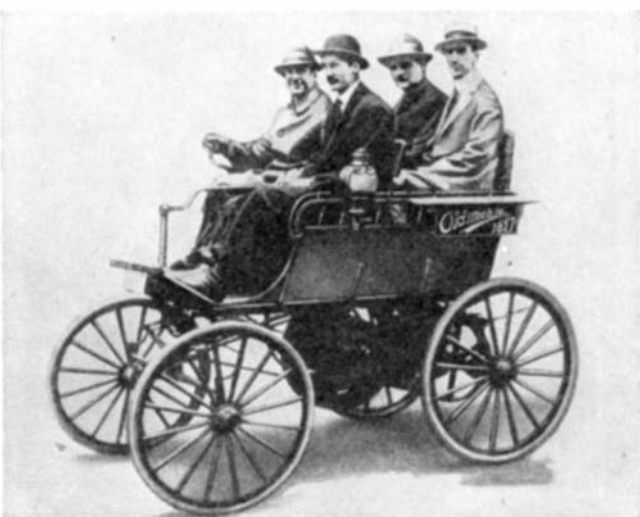
Most venerable of today's automobile is the Oldsmobile, which made its bow in 1897 with this single-cylinder model. A contemporary advertisement claimed a speed of 20 miles an hour on a smooth road. General Motors acquired Oldsmobile in 1908
