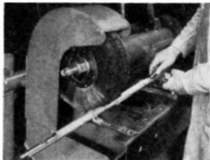
Two simple fixtures for power brushing. Above: A pipe holds threaded studs. Right: Forceps grip small parts
