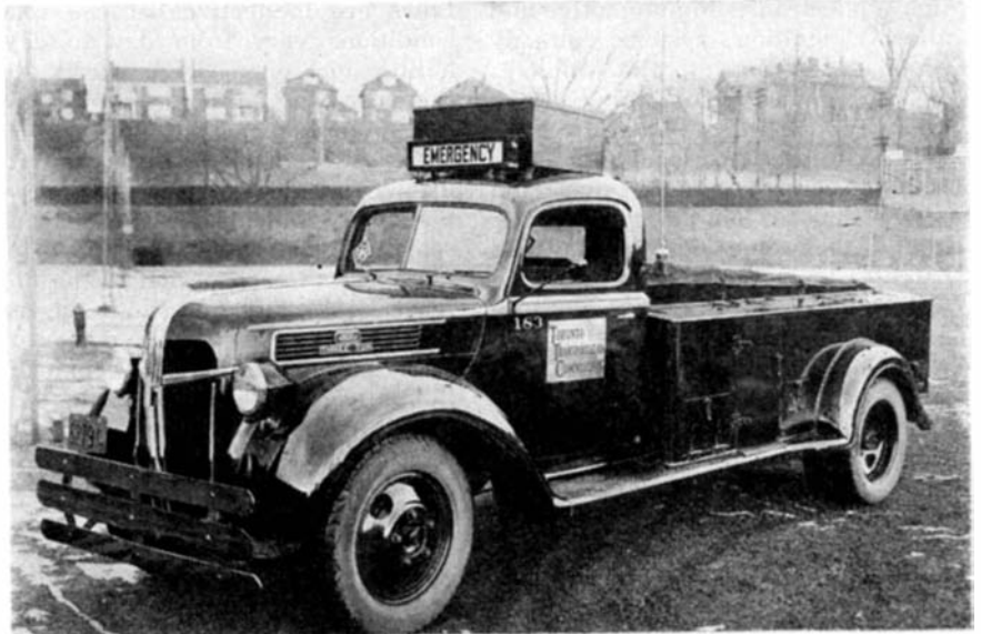
Emergency truck of the Toronto Transportation Commission, equipped for two-way frequency-modulation communication. In this installation the radio apparatus is on the roof of the cab and the antenna is alongside the driver
