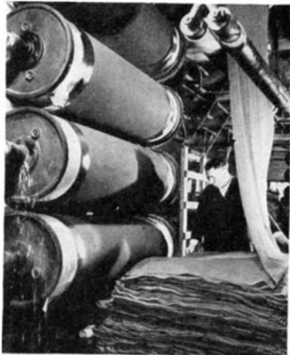
After impregnation and drying, new tent cloth passes through steam rollers (at top) and is ready for use
