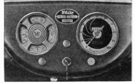
Instrument panel on a standard White truck showing how the "economy range finder" is built into speedometer dial
