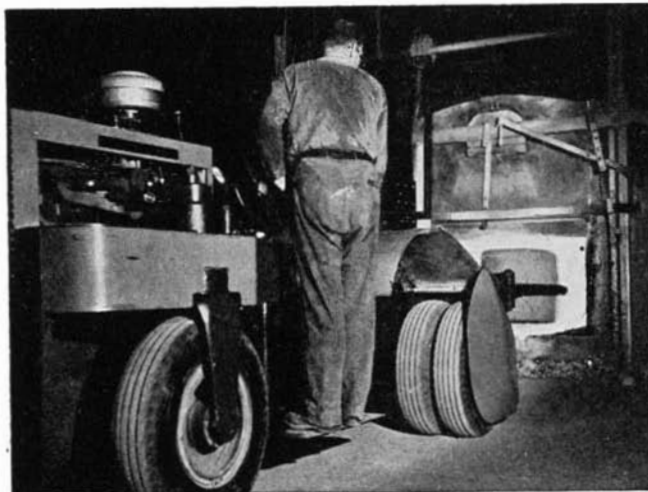
A modern pot-handling truck rolls on pneumatic tires, is completely mechanized, and is operated by one man
