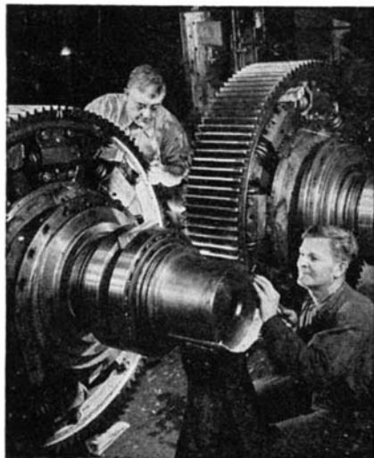
Driving-axle and main driving-gear assembly. When completed the cushion springs between the gear and the axle-spider arms will be enclosed
