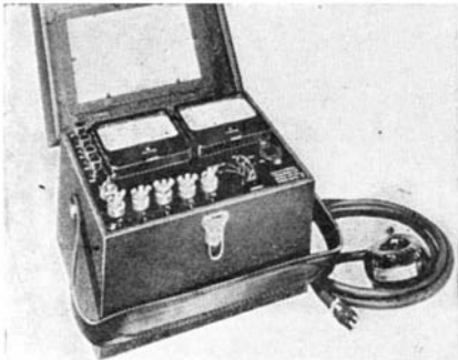
Double-purpose electrical meter for indicating both voltage and current
