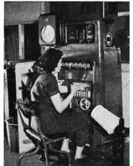
Setting up the cord tension vibrator which includes provision for determining effects of heat on cord life
