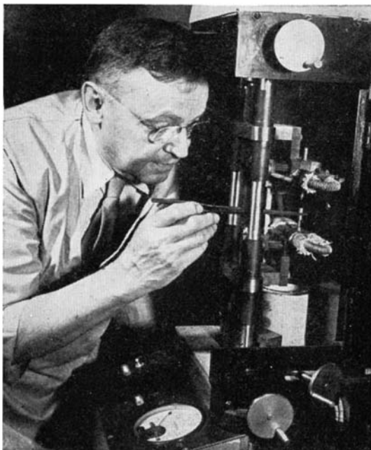
Dr. Rentschler, the author of the accompanying article, inserts (left) a carbon cup containing powdered glass into the lower jaw of the spectroscope's arc stand. It was in the course of such work that the cause of solarization of glass by ultra-violet rays was determined. Right: A close-up of a burning sample in the carbon electrode after igniting
