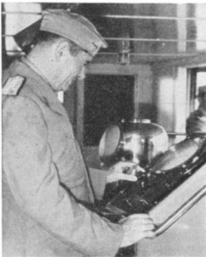
Left: Watching the screen of the electronic navigator, first peace-time version of war-time radar. Above: A photograph of the cathode-ray screen, showing how obstacles in the path of the ship are indicated. The operator can interpret quickly the kind of objects represented by the radar spots and their distance from the ship
