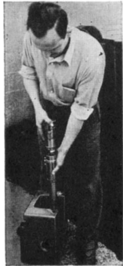
A portable instrument for making hardness tests. It does not require the services of a skilled operator and may be taken direct to the location where tests are to be made
