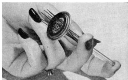
Steel header insert is sealed to the glass button through which wire leads are introduced into a vacuum tube
