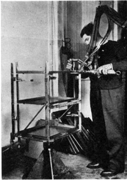
Assembly spot-welding of tables carried out with minimum of investment
