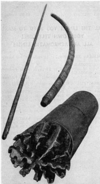
Left: Three units required in drilling a horizontal hole. A mandrel; a curved, flexible drill pipe; and a pressure operated turbine bit
