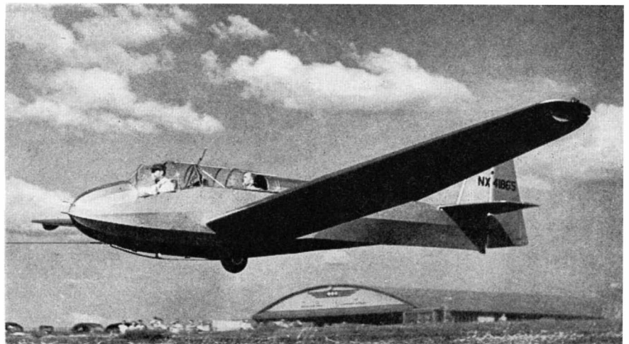
A towed glider leaves the ground; elastic tow line absorbs the initial shock
