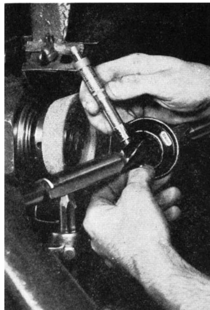
Blast nozzles of boron carbide, because of the hardness of the material, have extremely long life. In many cases, where ordinary nozzles will last only a matter of a half hour or so, a switch to boron carbide nozzles results in a life extension of some 3000 times
