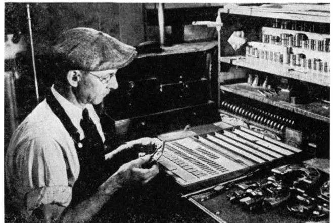
Standard gages, accurate within one millionth of an inch, are used as masters to check shop's production gages
