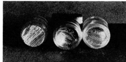
Localized molding of thermoplastics is successfully accomplished by use of frictional heat. The rough surface of the plastics (left) takes a perfect, clean impression (right) of the metal die shown in the center
