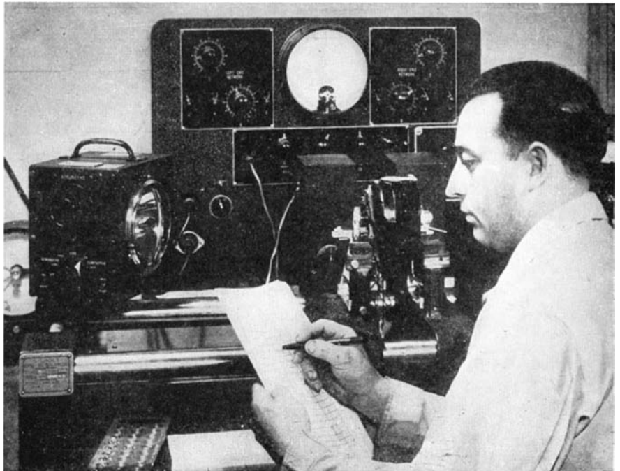
An electronic balancer, combined with a stroboscopic light to measure speed of rotation, detects the amount and location of unbalance in a rotating part
