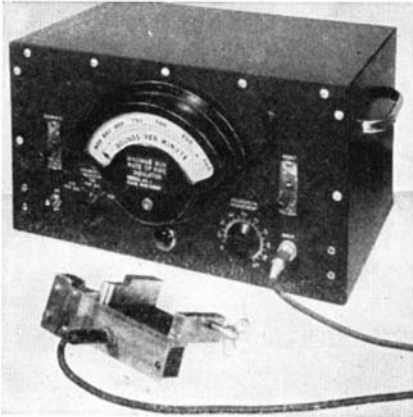
Operating rates of machine tools, or other rapid-moving equipment, may be readily checked with an adaptation of this electronic gun-fire rate tester
