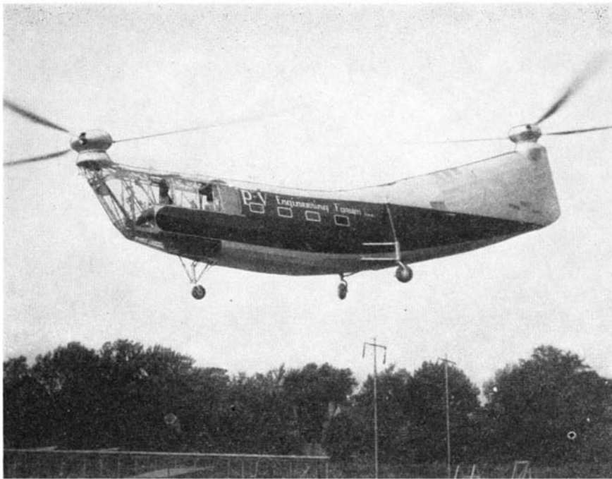
Progressive helicopter designs, such as the PV-2—10 passengers and 110 miles per hour—bring fast local service and short inter-city air hauls nearer reality
