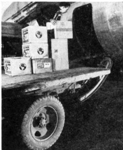
Truck-level cargo doors save handling; are partial answer to loading problem
