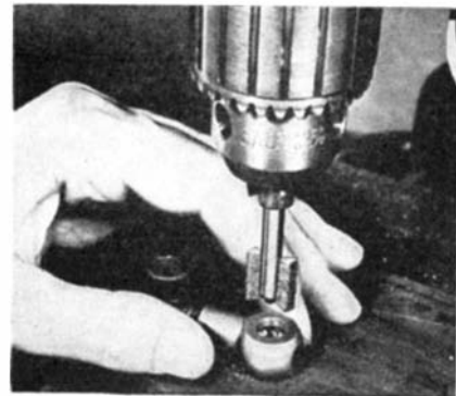
Above: Simultaneous brushing of two inside diameters. Below: Removal of drilling burrs from intersecting holes in "hard-to-reach" spot in small part
