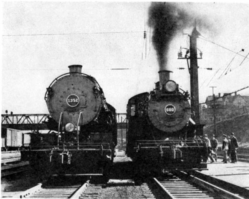
Locomotive at left is using new over-fire air jet; one at right is not
