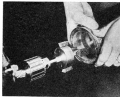
Above: Simultaneous brushing of two inside diameters. Below: Removal of drilling burrs from intersecting holes in "hard-to-reach" spot in small part
