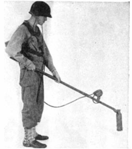
Portable mine detector spots metallic or non-metallic sub-surface objects; headphones and meter signal a pickup
