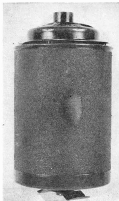
Remarkably clean, this oil filter was operated 300 hours on detergent oil
