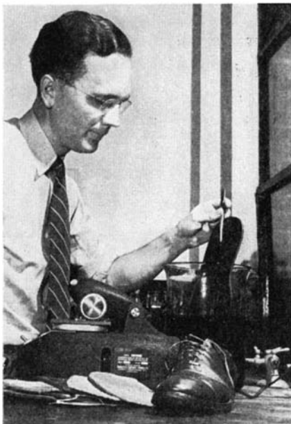
Life of sole leather is upped about 25 percent by processing with special oil. Abraser in foreground tests soles
