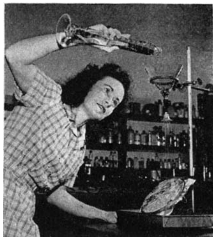
Photographs courtesy Socony-Vacuum Testing a wax-emulsion-treated fabric for water repellency. Cloth remains porous, but water runs off its surface
