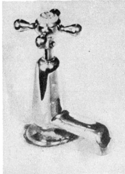
Service testing, on such articles as faucets, proved speculum's durability
