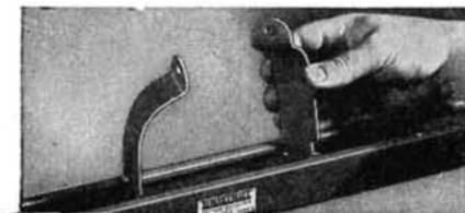
1 How cable clamp straps are inserted.
