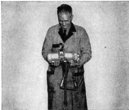
Lightened by aluminum housing design, portable half-ton hoist is easily carried or installed by one person
