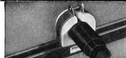
3 One bolt tightens clamp, locks it to support.
