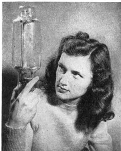
Inner quartz tube houses arc stream at four times previous vapor pressure. Lamp will burn in any position
