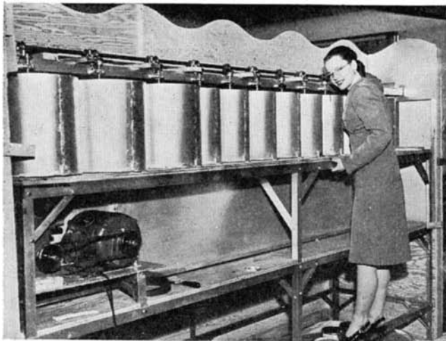
Front (right) and rear (left) of color dispenser to speed mixing of basic paints; motor driven agitators ensure pigment suspension
