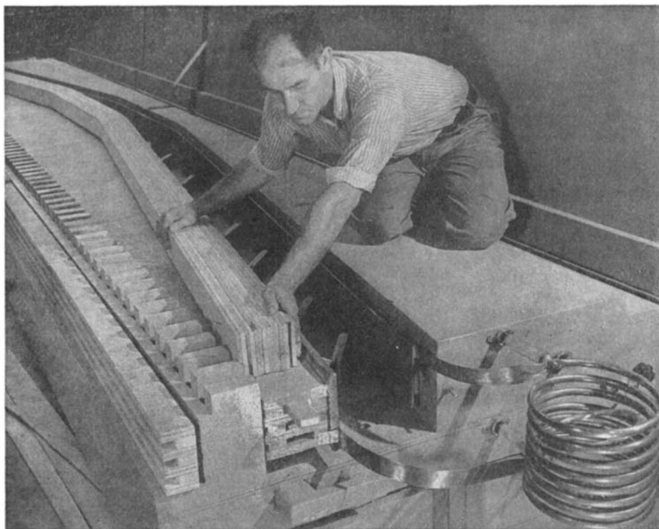
Laminated spar flange for a Fairchild airplane being removed from press. Here high-frequency energy simultaneously molds the wood and sets the glue quickly
