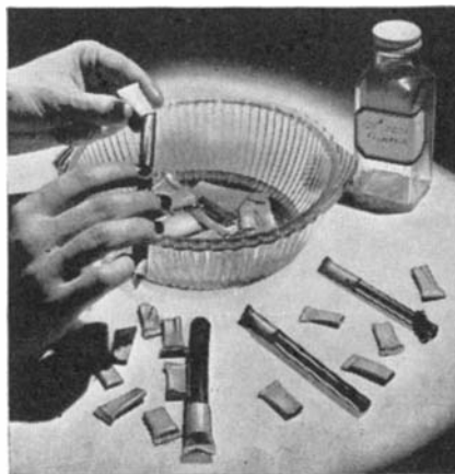
After soaking five hours in dilator, seals slip on easily, shrink to fit
