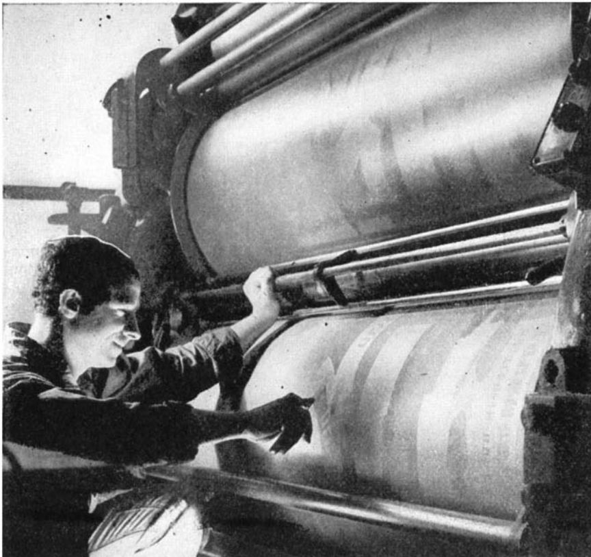
Synthetic rubber for printing rolls takes large proportions of plasticizer oils
