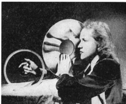
Lens-mirror combination for television receivers. The mirror (center) distorts the image; the Schmidt lens (left) corrects the mirror aberrations
