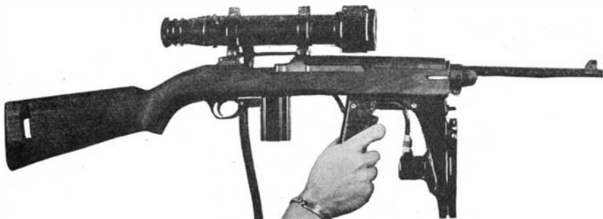
Sniperscope, American night gun, mounts infra-red light and scope on a carbine
