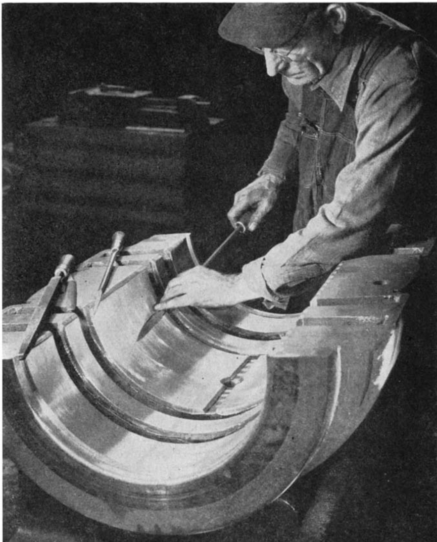
Hand-scraped bearings still hold their own on many important jobs in industry since their characteristics have been proved through long and successful use
