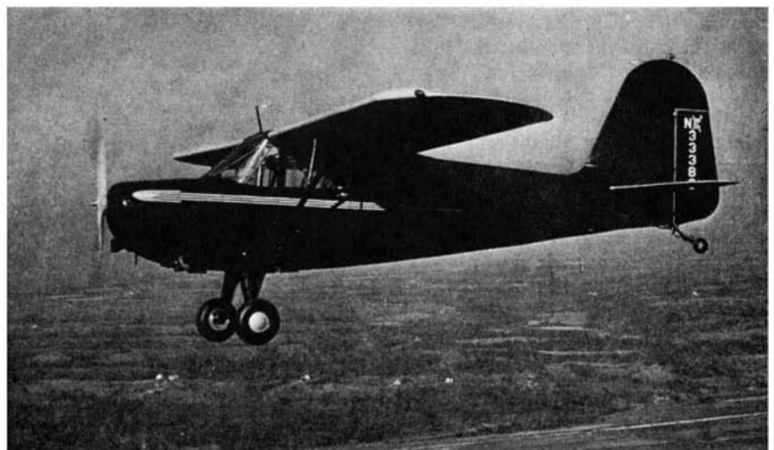
Range of 600 miles and wing slots are Skyraider safety features
