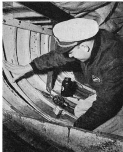
Repairing a boat by use of gap-filling glue and laminated ribs. Left: The glue is applied to the surface of the first ply, which was cold-bent to shape and screwed in place. Above: The second ply is bent and fastened
