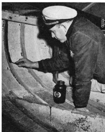
Repairing a boat by use of gap-filling glue and laminated ribs. Left: The glue is applied to the surface of the first ply, which was cold-bent to shape and screwed in place. Above: The second ply is bent and fastened
