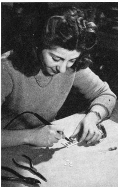
Miniature tube leads are soldered to printed circuit; wires are eliminated
