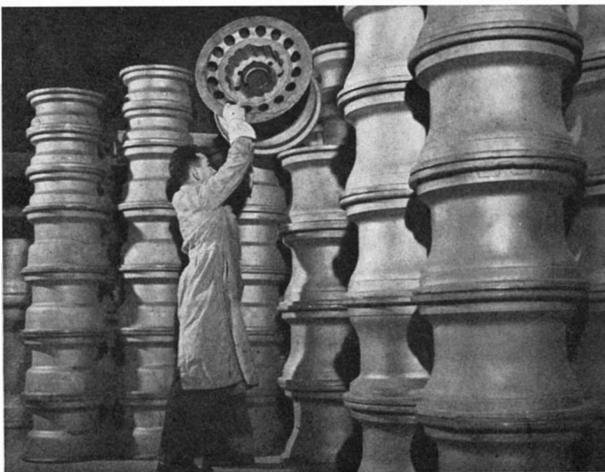
Light enough for one man to handle, magnesium aircraft wheels carry heavy loads
