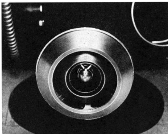
Combustion head installed in blower mouth. For best efficiency, relative positions of oil nozzle, flanges, and blower mouth are mutually adjustable
