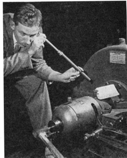
Tube length is adjusted to resonant wavelength of turbine "trouble" noise
