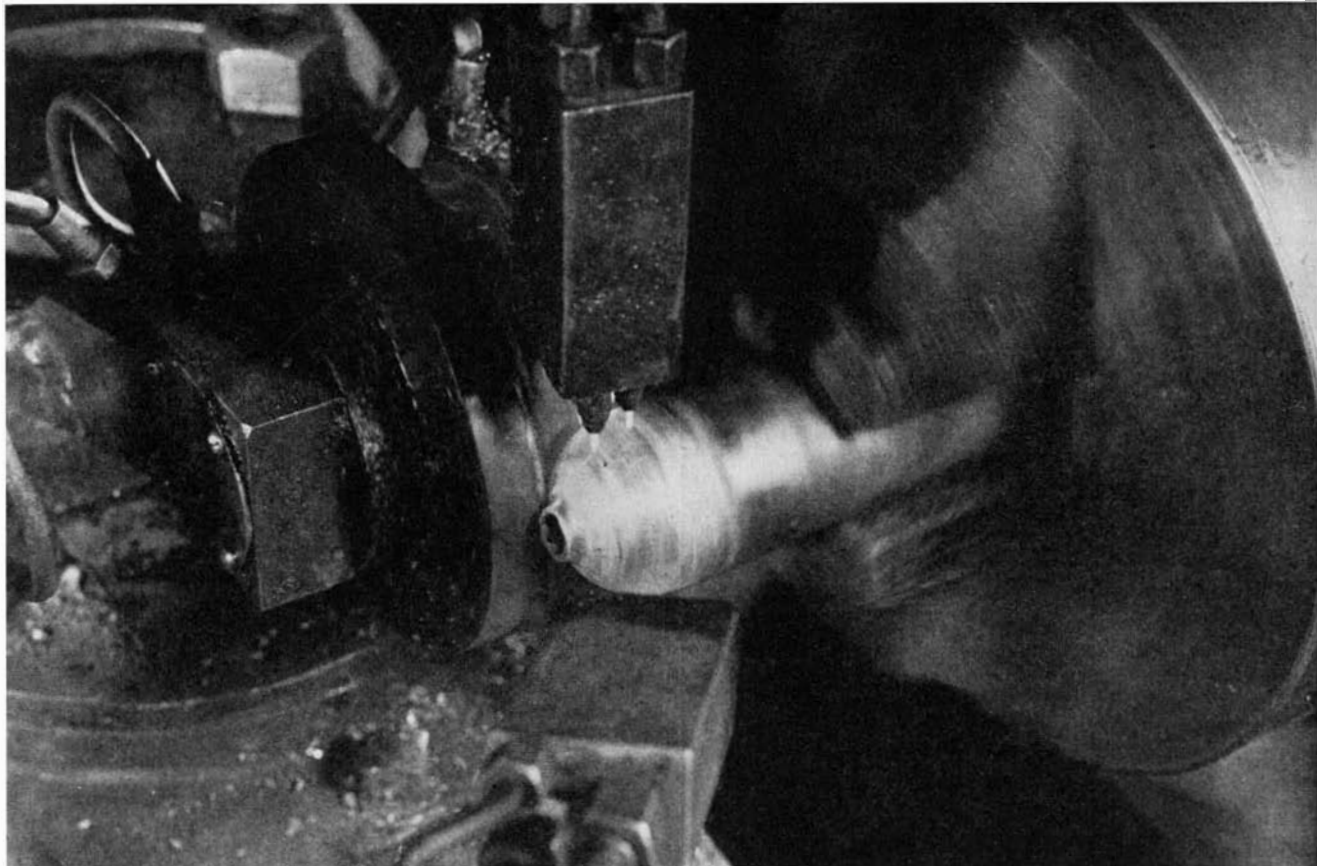
Oxy-acetylene flame spinning, supplanting deep drawing for many operations, will close tubing ends or reduce diameters at any point. Practicality of such methods requiring intensely hot flames depends to a large extent on low-cost oxygen of highest purity
