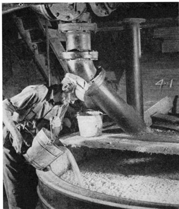
Wax treatment of paper is often done after the paper is manufactured. Here, however, a wax-emulsion sizing is added to pulp in beater to impart water resistance to, and lay surface fuzz of, finished paper
