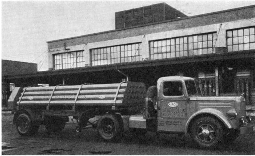
Large, multi-tank trailers are connected to plant oxygen manifolds—usually two trailers are used, one as a standby. Such equipment boosts oxygen uses
