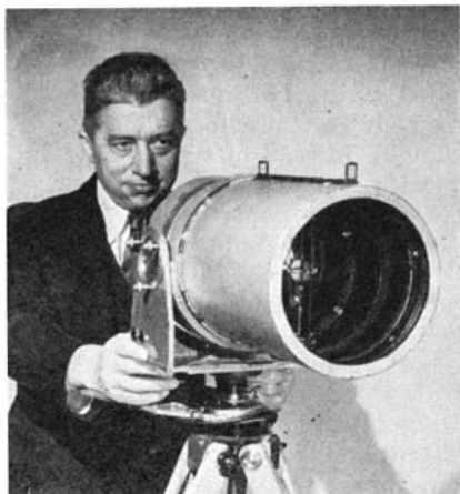
Thermistor-type bolometer can detect man's body heat at quarter-mile range
