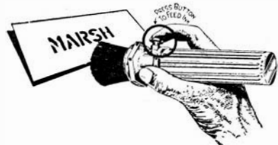
Finger-tip button controls ink flow
