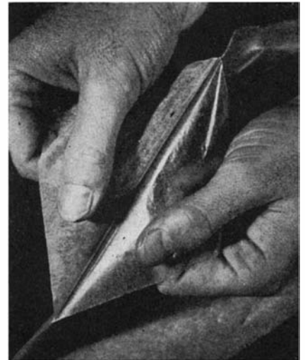
Wax between layers of paper laminates acts as adhesive and moisture barrier
