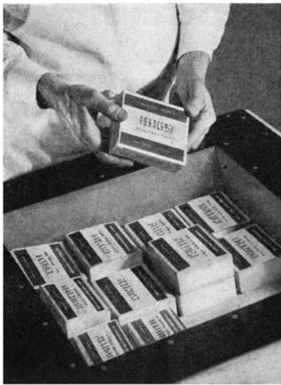
Microcrystalline waxes stay flexible at low temperatures, do not chip or flake in packaging of frozen foods
