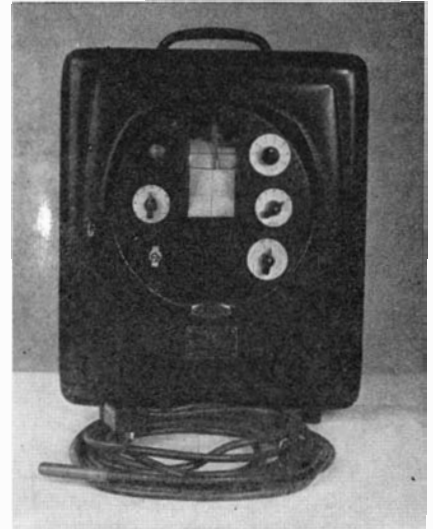
Probolog is compact, easily carried to job. Pen traces permanent record
