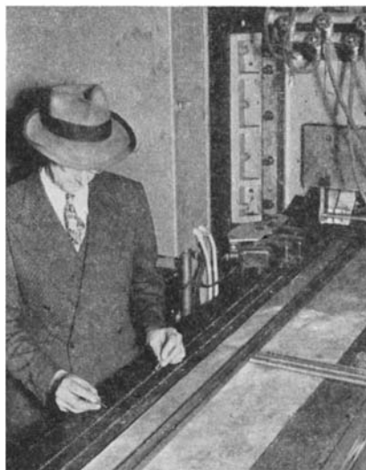
Placement of light-blocking rivets (above) controls welding positions. Full view of welding machine (below) shows 10- by 30-foot traveling table
