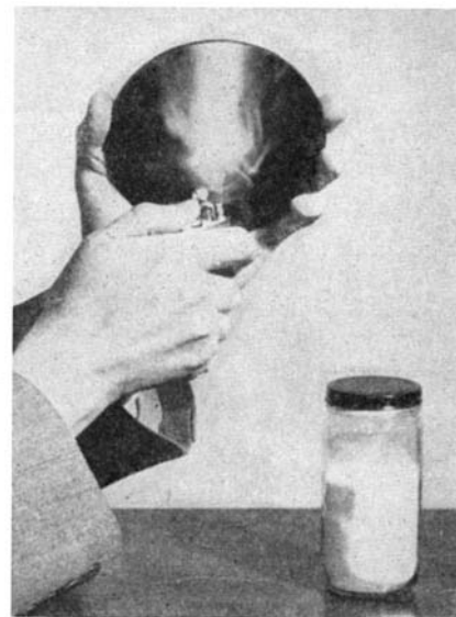
Ethyl silicate burns to give a white deposit of fumed silica on the plate
