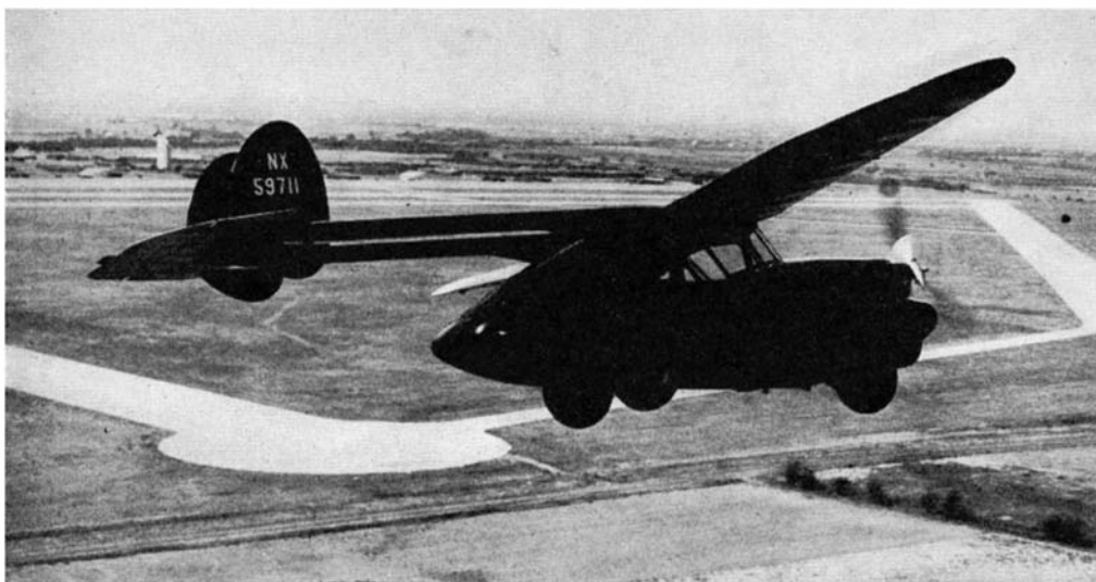
Roadable plane, still experimental, matches popular concept of what such a craft should be on most points—price excepted. Wing-tail unit and propeller are taken off at airport; a mechanic must reassemble them to body before next air trip
