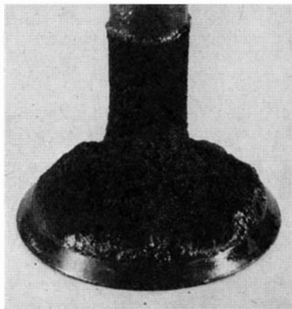
Dirty valve (above) and piston (below) compare with relatively clean valve and piston to demonstrate the importance of selecting proper fuel for a given engine
