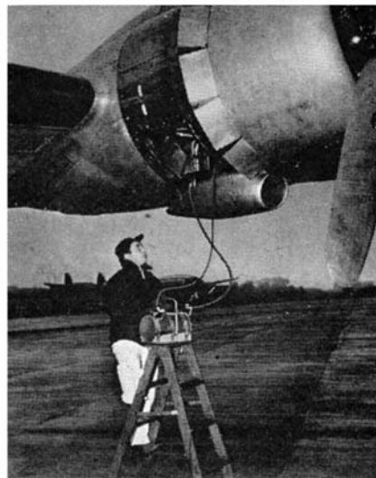
External tank connected for starting
