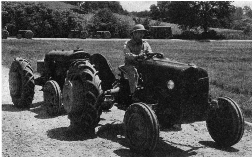
New tire tread on front tractor outpulls older tread on tractor being towed
