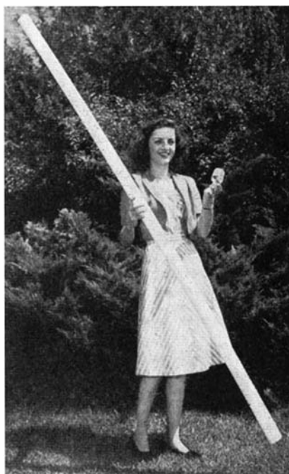
Individual cell walls seal out water, prevent insulating plastics freezing on inside. Girl holds equal weights of solid and expanded Styron plastics
