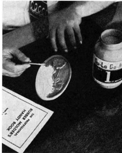
First step in making mold: spreading mixture over object to be reproduced
