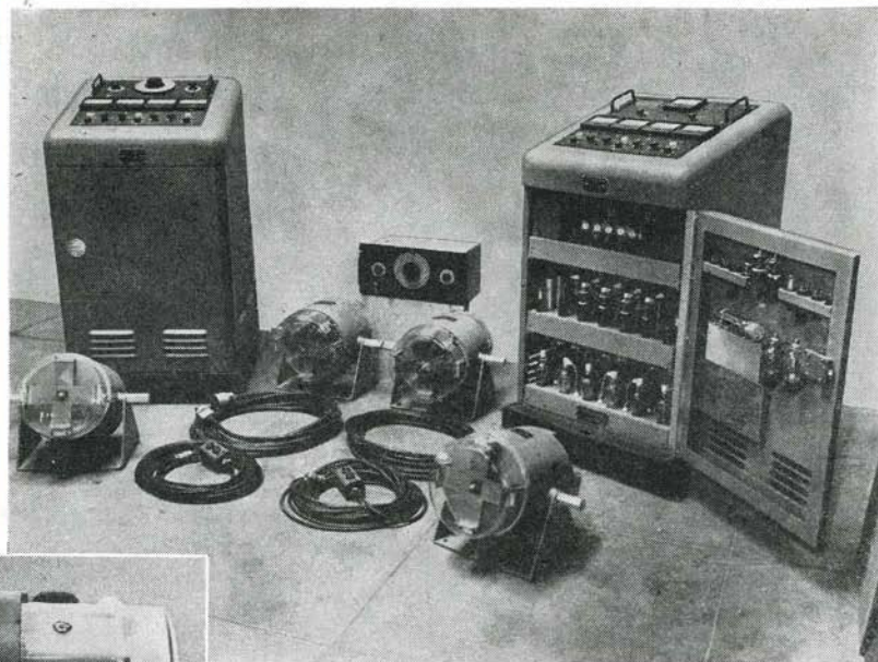
Electronic equipment in cabinets (above) will drive shakers on floor over a wide frequency-amplitude range. Shaker unit (left), is basically similar to a radio loudspeaker
