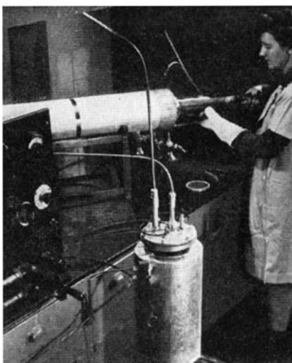
Operating on a laboratory scale, this Harshaw model cell supplies fluorine for reaction in an electric furnace
