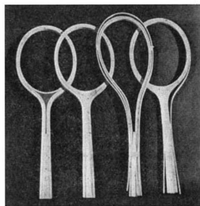
Racquet frames used in glue tests
