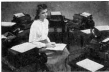
Guided by holes in tape, letters are typed automatically, leaving the operator free to check her mailing lists
