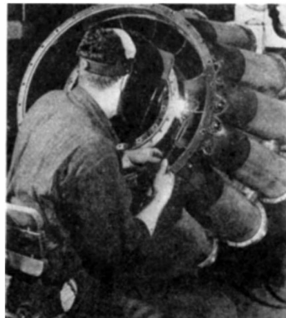
Alloys welded in hydrogen atmosphere
