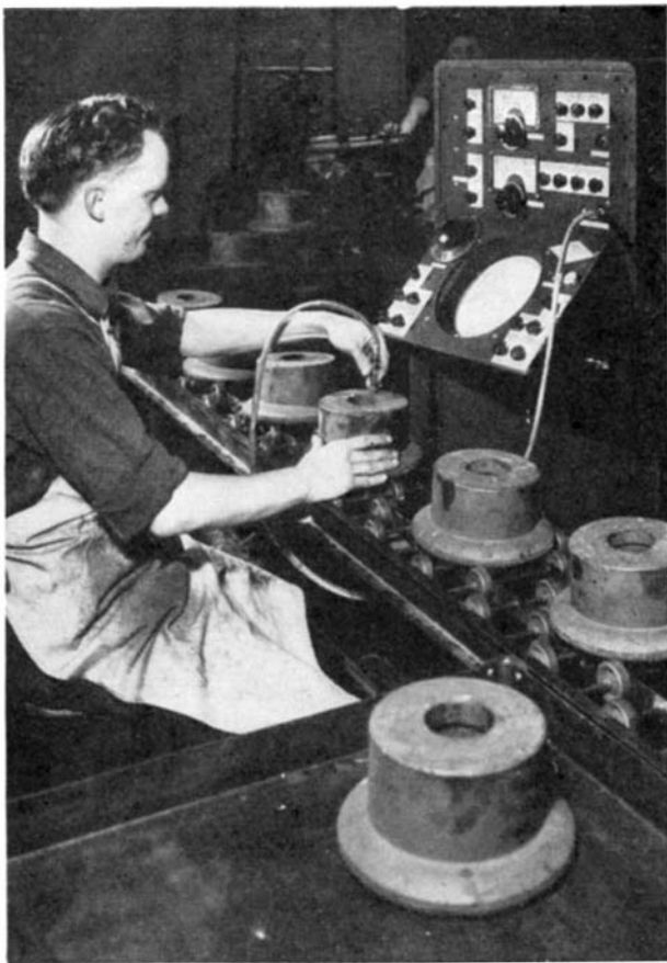
The Reflectoscope sends supersonic waves through the castings (left). A flaw's presence is revealed on oscilloscope screen by pip, D, on trace (lower right). If the piece is not defective, trace (upper right) is undisturbed
