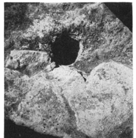
Above: Blowpipe coming out of hole at end of run. Below: A six-inch blast hole produced by fusion piercing
