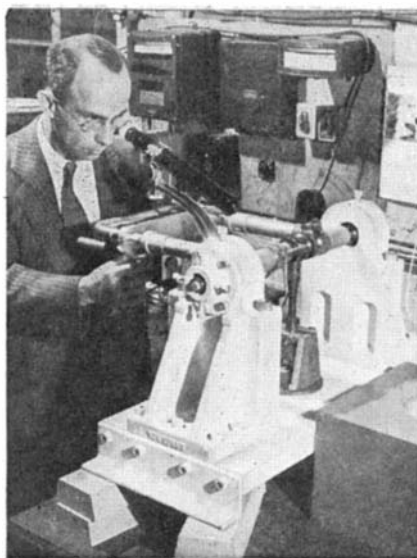
Tuned air column can produce stresses up to 100,000 pounds per square inch
