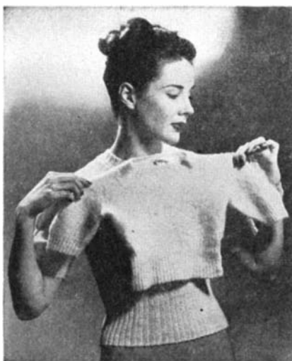
Sweaters, originally same size, were laundered in same manner; untreated one shrunk, Koloc-treated one did not
