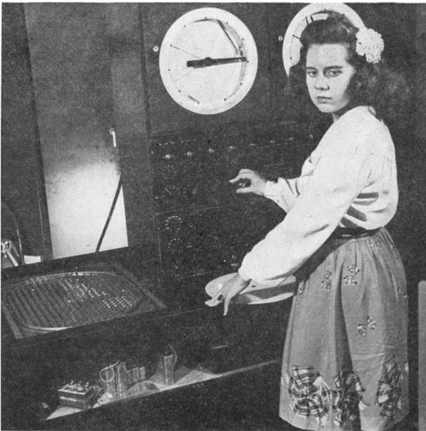
With all the necessary information applied to the analyzer's control panel, the machine will simulate, on a miniature time base, the changes that would occur in an underground reservoir, represented by the circular tray at extreme left
