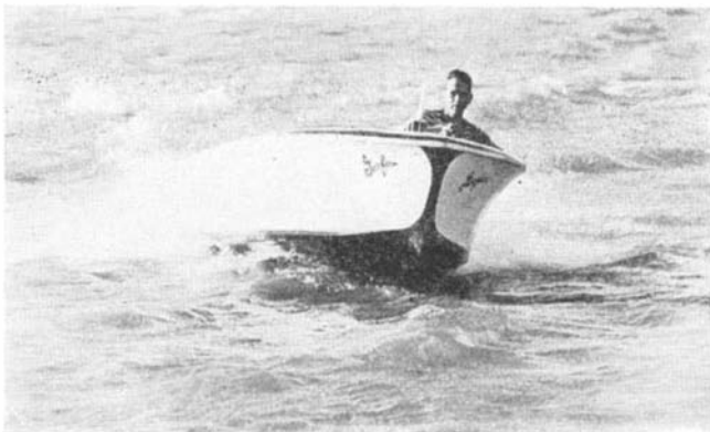
Made in one seamless piece, the seaworthy utility craft demonstrates its maneuverability at full speed
