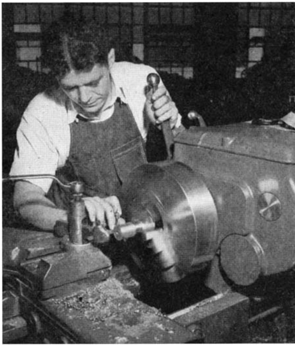
Carbide tools, when first developed, were easy to use with manual control. But the carbide family had to multiply before the tools could be successfully applied to automatic and integrated machine control
