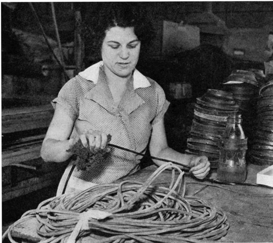
Wiping finished rubber tubing with glycerine helps prevent drying out
