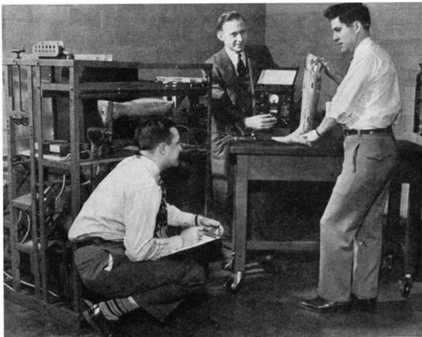
Fatigue tester, shown at left, compresses three years' walking into ten days
